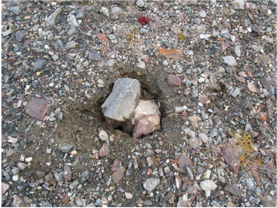
Photo: 15: Vent raise subsidence filled with waste rock.
