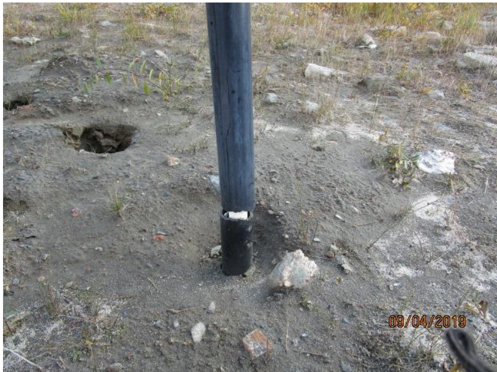
Photo 18: Thermistor T-4 casing damage.
