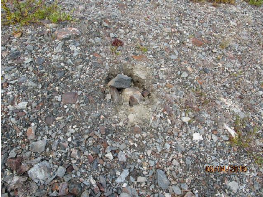
Photo 11: Small area of subsidence at B-zone Vent Raise.
