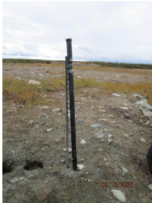
Photo 26: Thermistor T4 repaired and support with t-bar.
