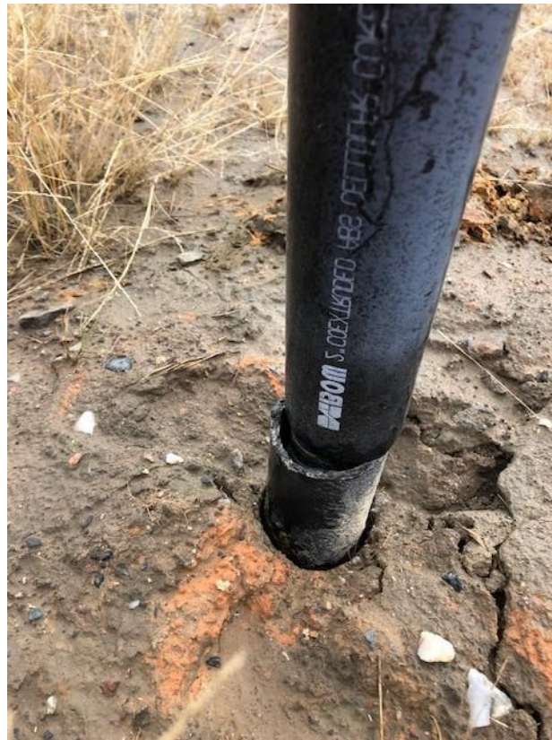
Photo 22: Thermistor T-1 example of casing damage.
