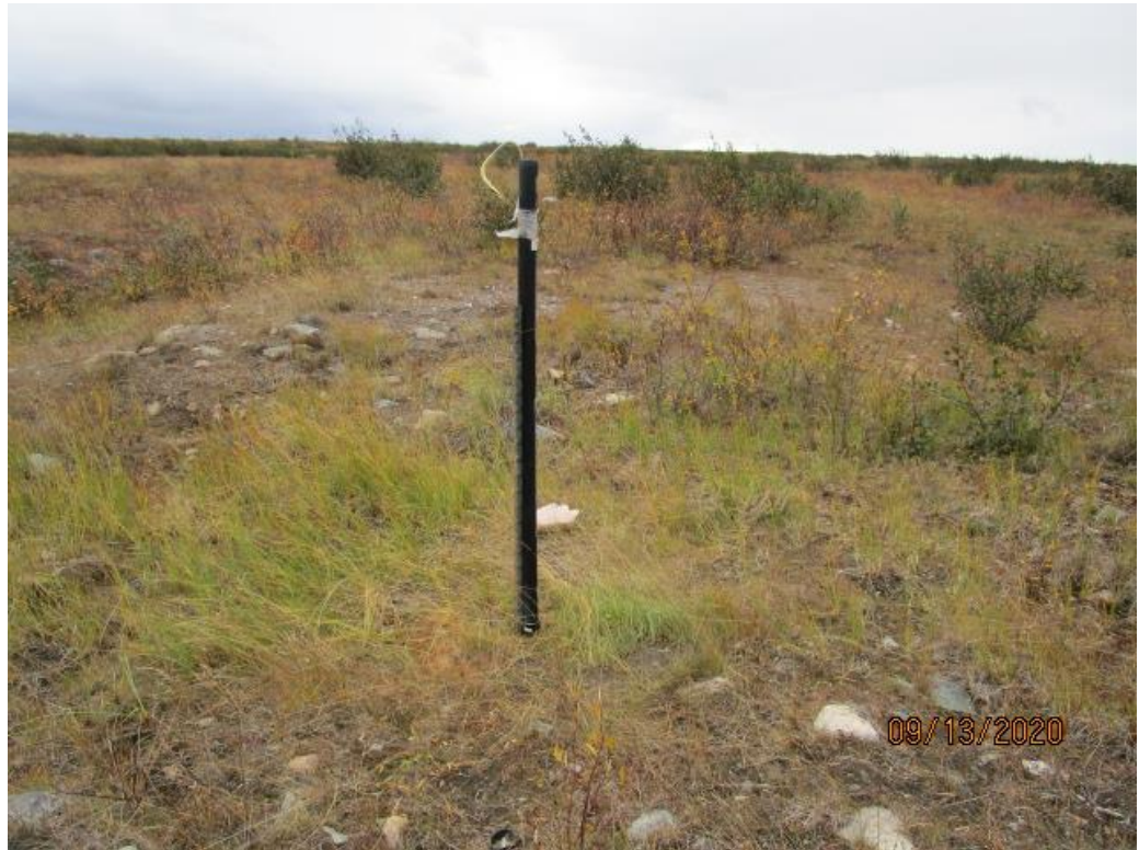
Photo 25: Thermistor T3 repaired with joiner at ground level.
