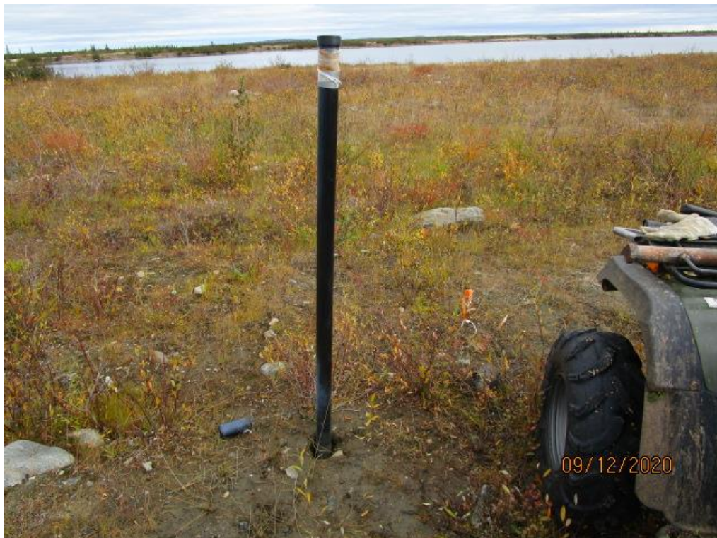
Photo 24: Thermistor T2 repaired with joiner at ground level.
