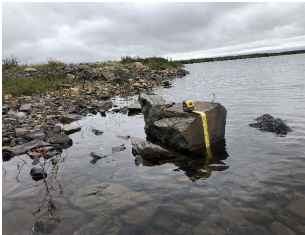
Photo 12: Tailings Pond No .1 reference for water level at spillway (Renate Klassen photo).
