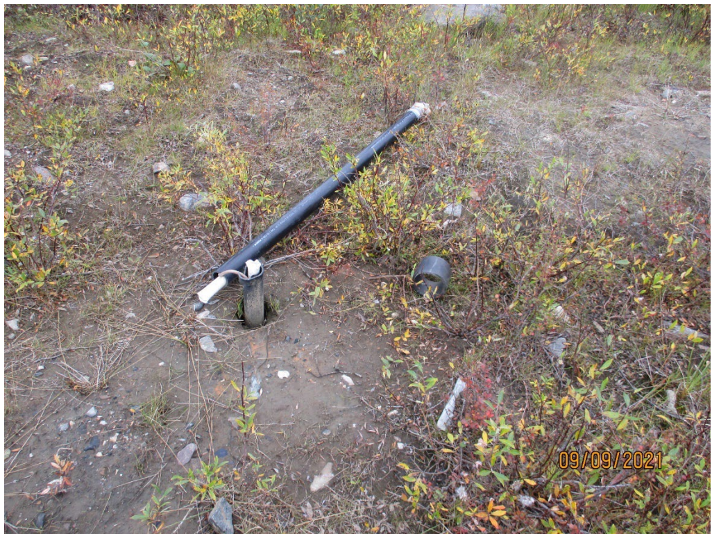
Photo 18: Thermistor T-2 casing damage.
