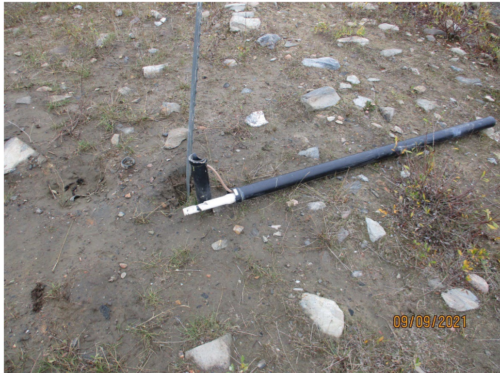
Photo 19: T3 thermistor casing damage.
