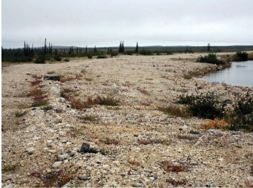
Photo 3. Faint evidence of oxidation of waste rock (yellowing).
