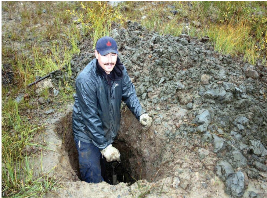
Photo 22. Excavation to permafrost depth showing unoxidized gold tailings (grey colour).
