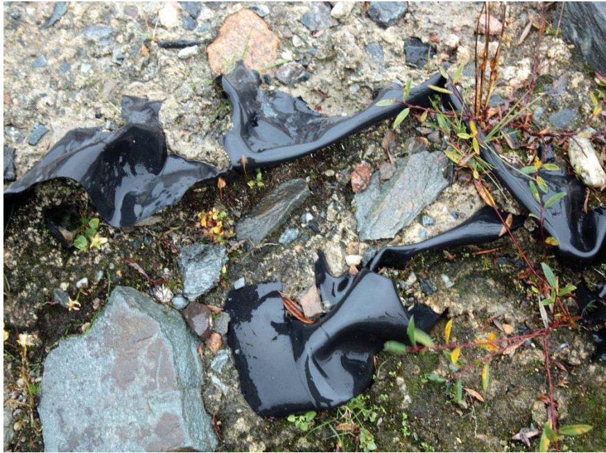
Photo 13. Shreds of liner dumped with spoil obtained from wall of TP2, to cover tailings in TP1.
