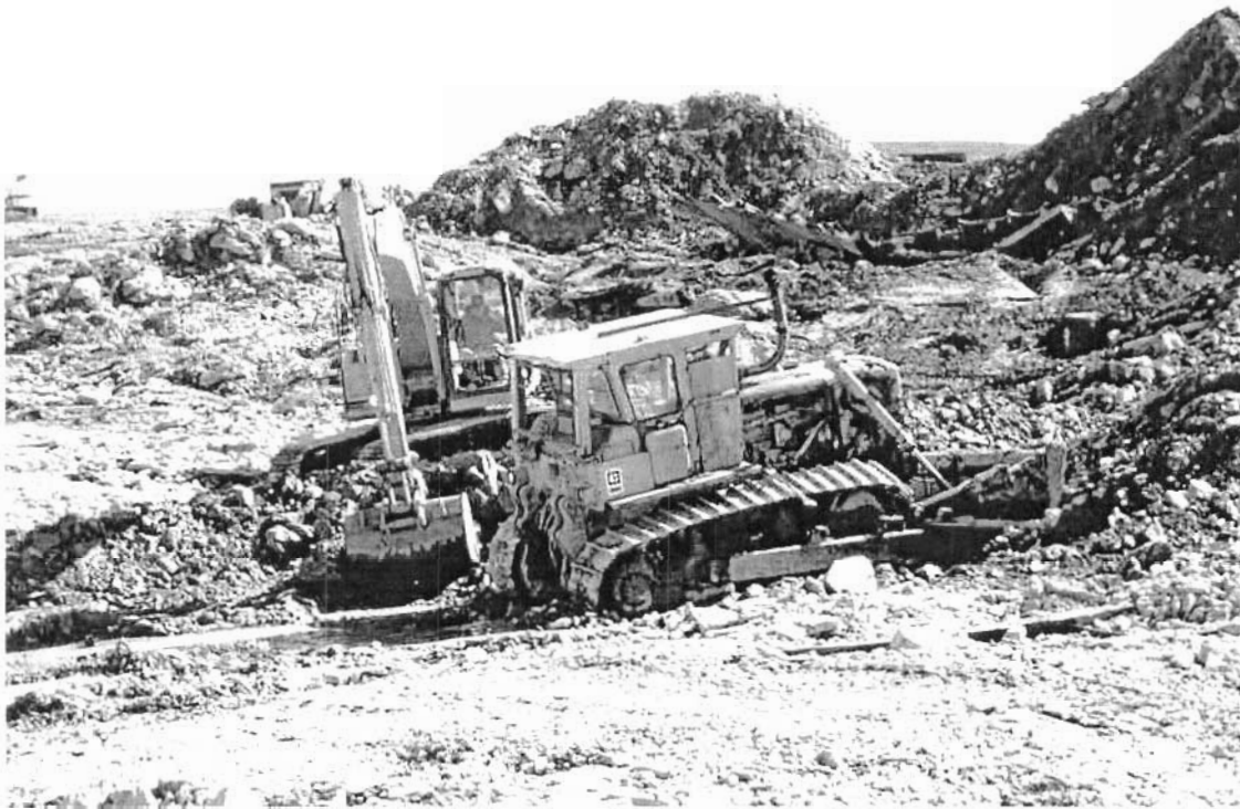
Dozer and Hoe flattening scrap material
