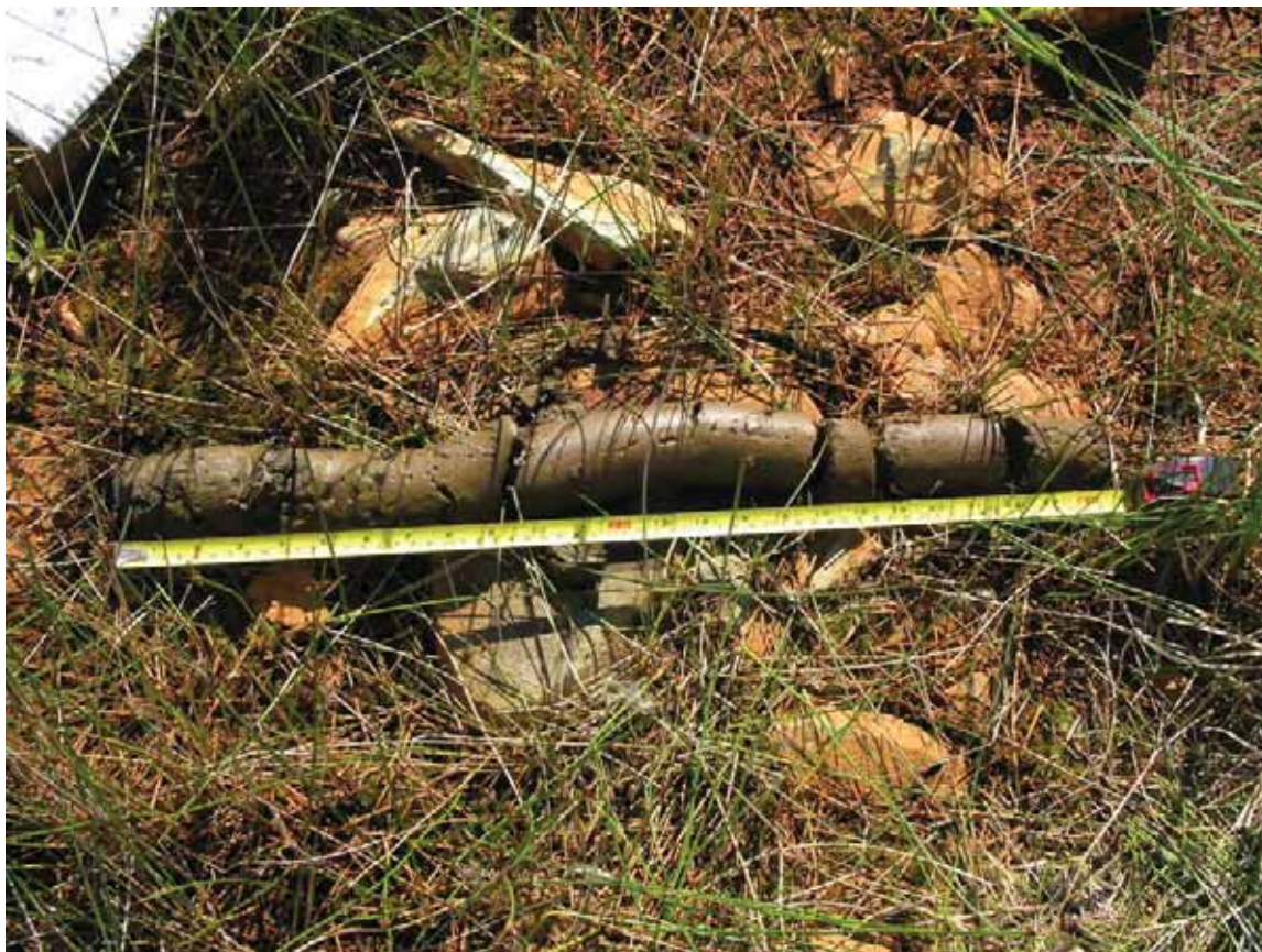
Figure 2-7: B-Zone Tailings Material Collected from MW-2.
