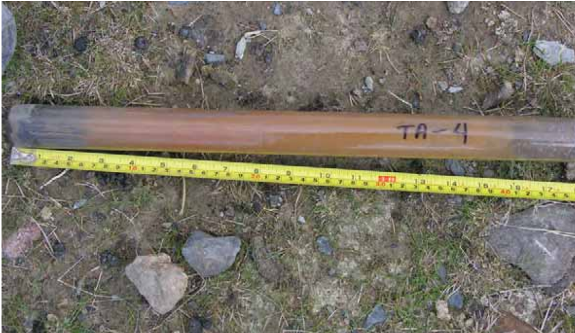
Figure 2-5: Example of Tailings Core Collected at Station TA-4 Prior to Freezing. Reddish Brown Tailings Indicate Shear Zone Material Between 6 cm and 40 cm. Dark Grey B-Zone Tailings at Base of Core; Till Material is above 40 cm.
