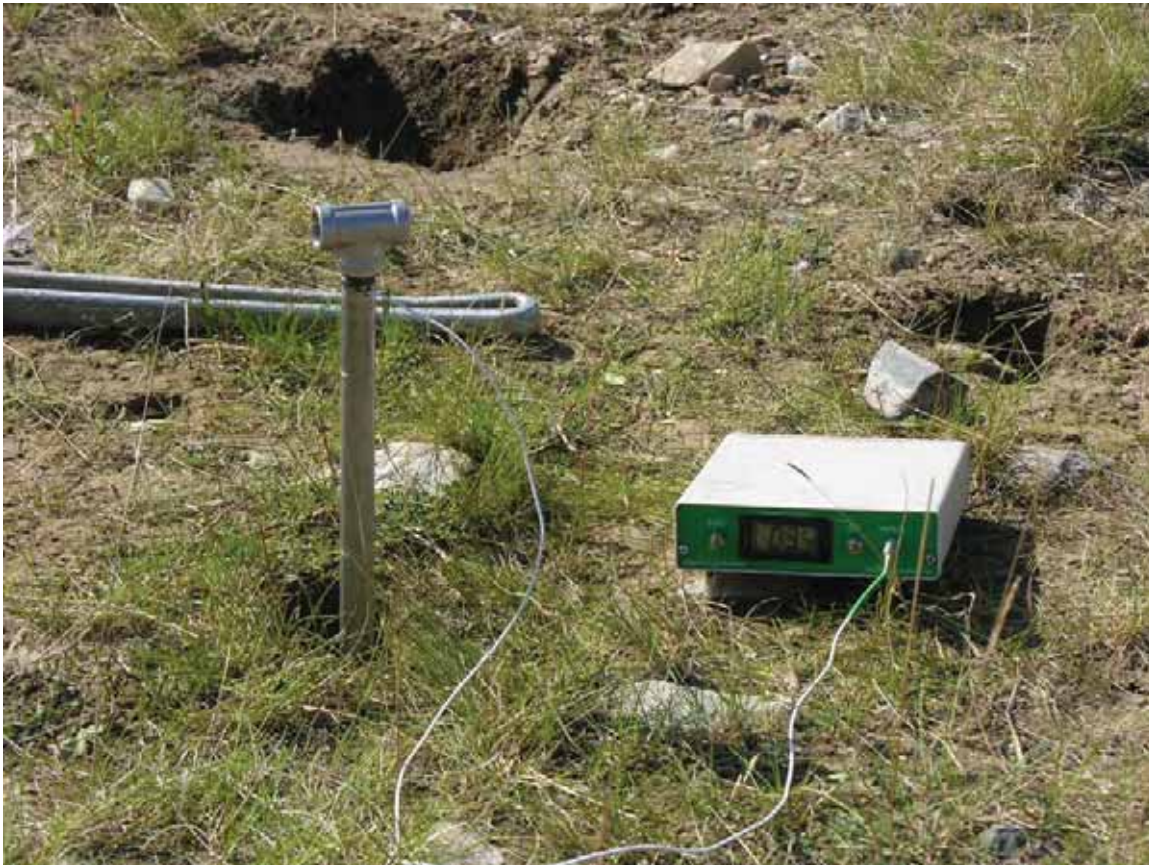
Figure 2-9: Set-up of Oxygen Meter Profile Apparatus
