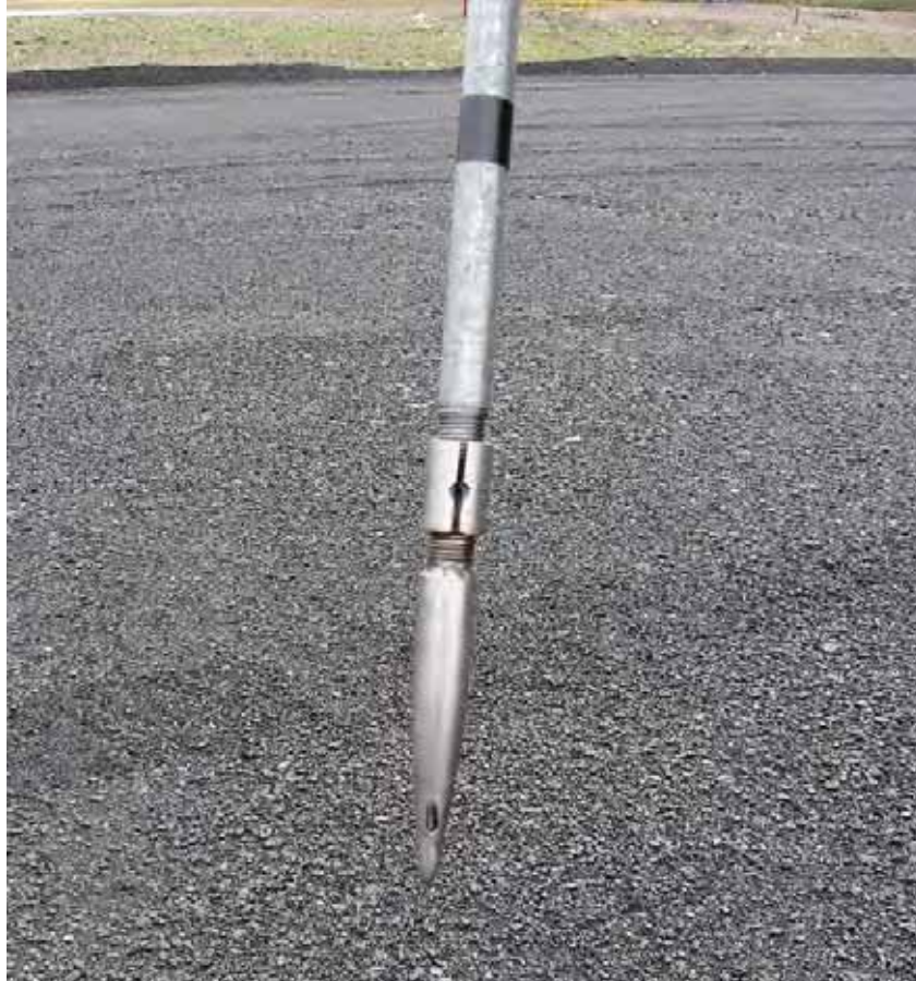
Figure 2-11: Tip of Mini-electrode Assembly
