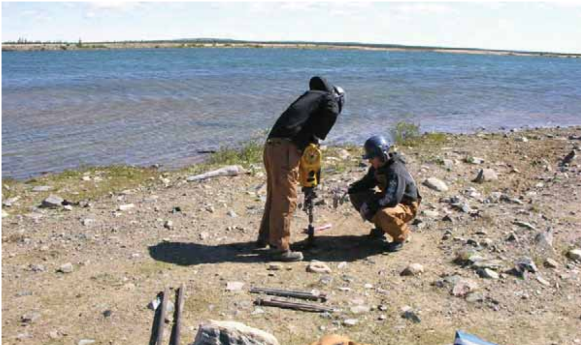
Figure 2-4: Operation of Pionjar Core Sampler at Station TA-1 at the Tailings Impoundment
