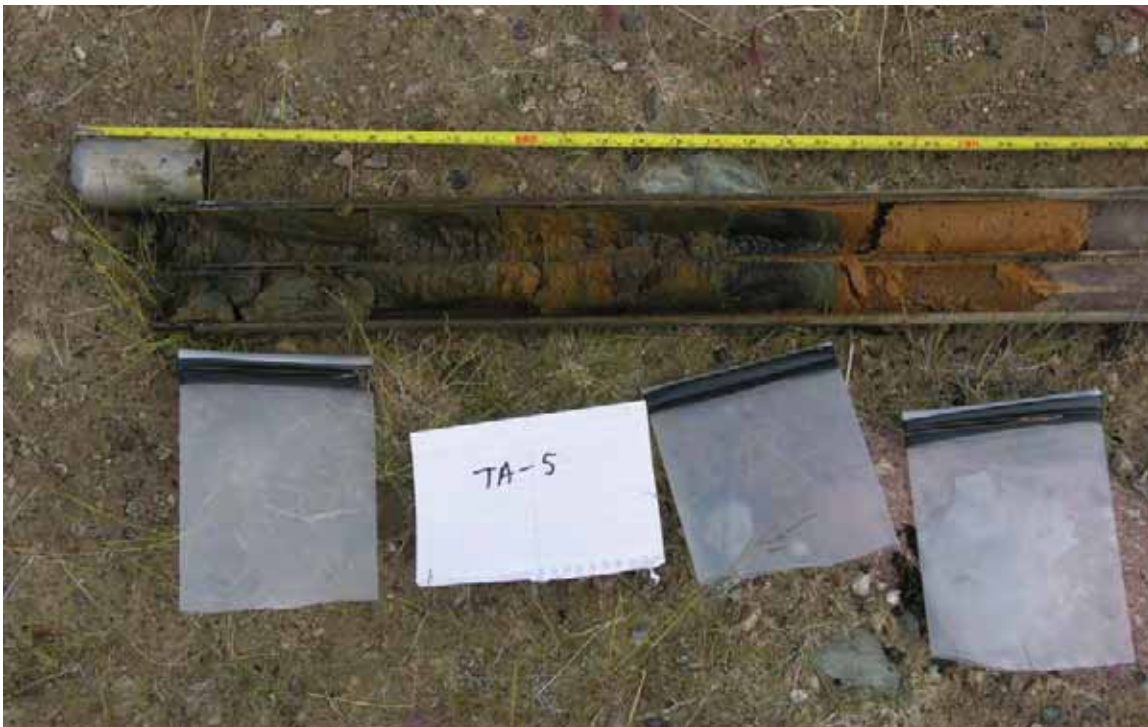
Figure 2-6: Example of Tailings Material Collected with Split-Spoon Sampler at TA-5. Shear Zone Tailings are Visible as Reddish Brown Tailings.
