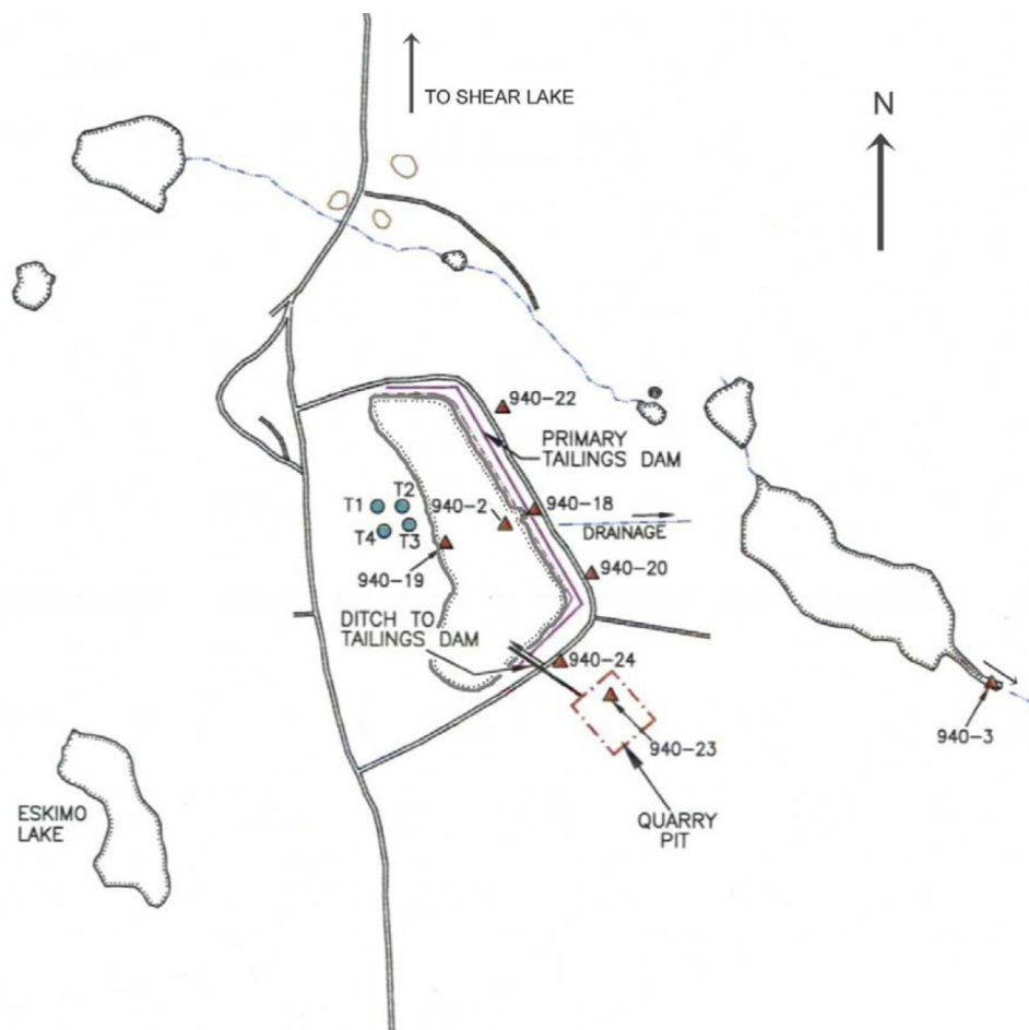
Figure 5-6. Location of Quarry Pit (map not to scale), thermistor (T circles) and water sampling (940-X triangles) stations.
