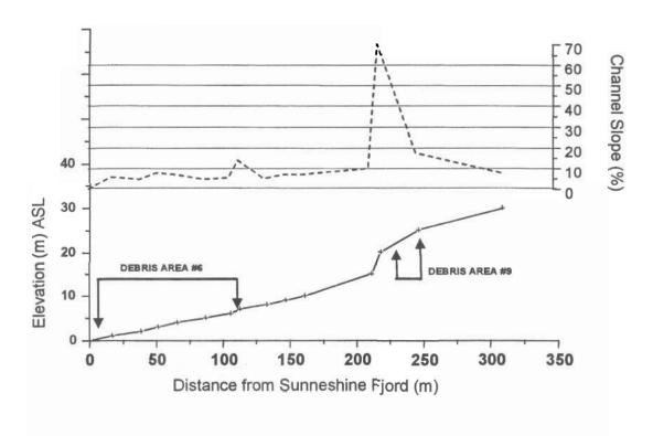
The extreme slopes of the streambed (>20% rise over run) at a distance approximately 200 m inland likely preclude the upstream migration of arctic char. For any particular stream reach, the streambed slope is expected to exert significant control over the hydraulic and biological characteristics (Montgomery and Buffington, 1993). For a temperate environment, Montgomery and Buffington (1993) noted the following slope – stream channel correspondence:
