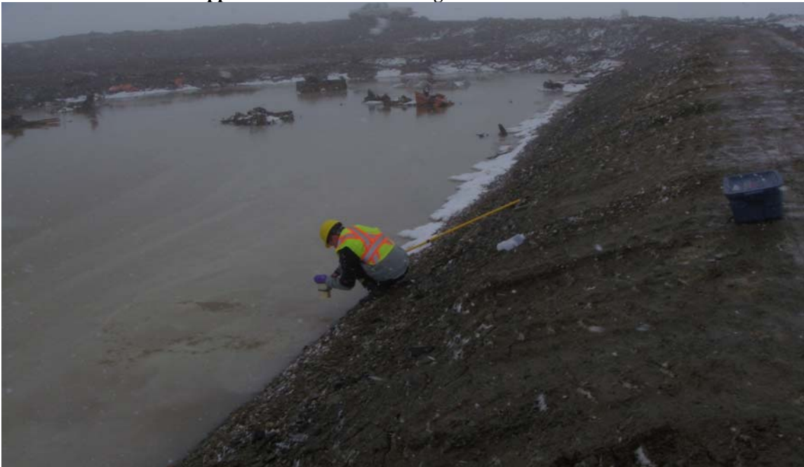
Photo 6 (DCS01155): Sample 09-50054 collecting a wastewater sample from ponded water in the northwest corner of the Upper Site. Photo taken facing south.
