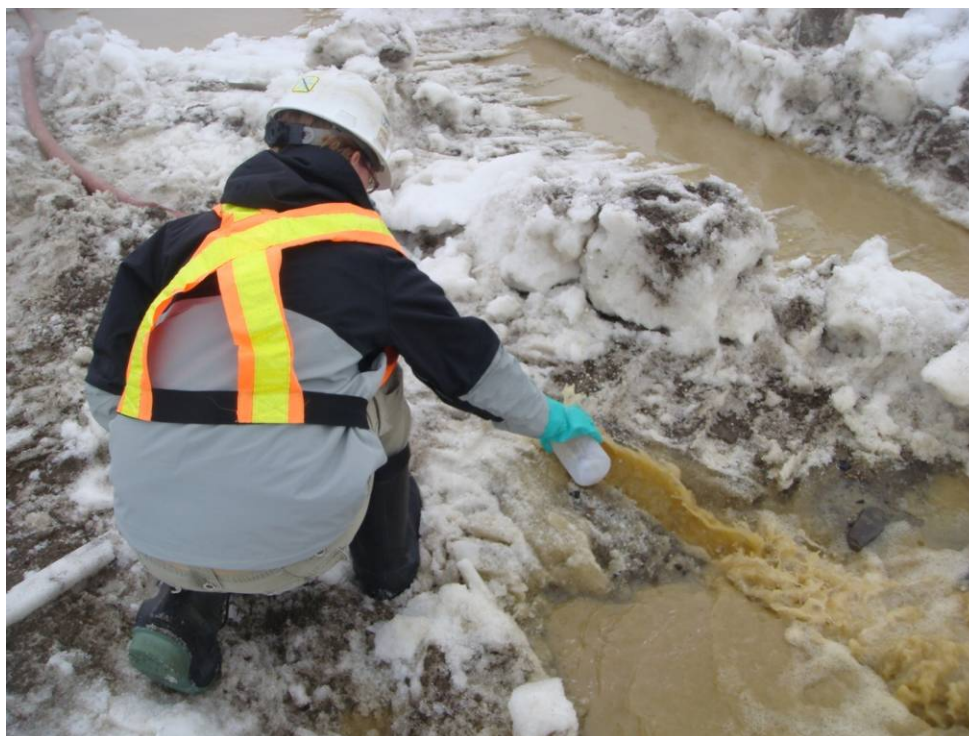
Photo 5 (DSC01027): Sample 10-21245 Dye-M Collecting a wastewater sample from the pump discharging water from the landfill
