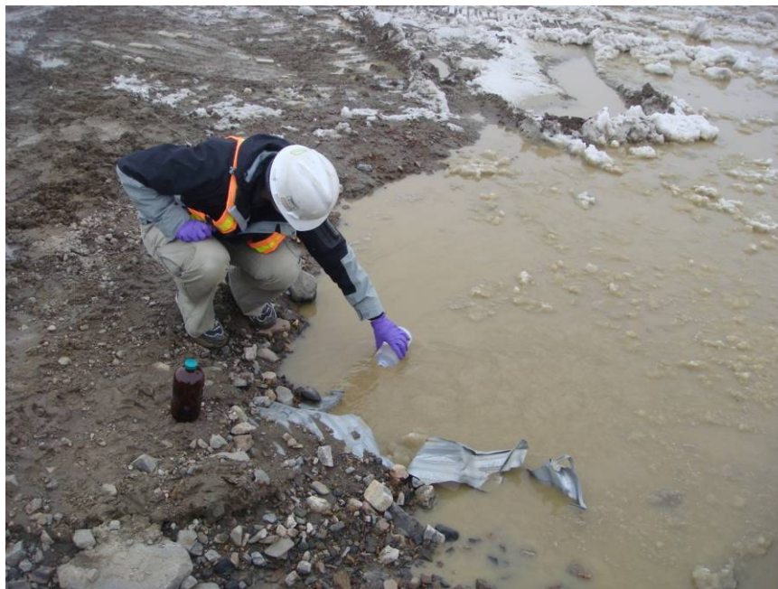
Photo 6 (DCS01028): Sample 10-21246 Dye-M Collecting a sample from culvert downstream of landfarm discharge - Northeast culvert at crossroads (MPA 4)
