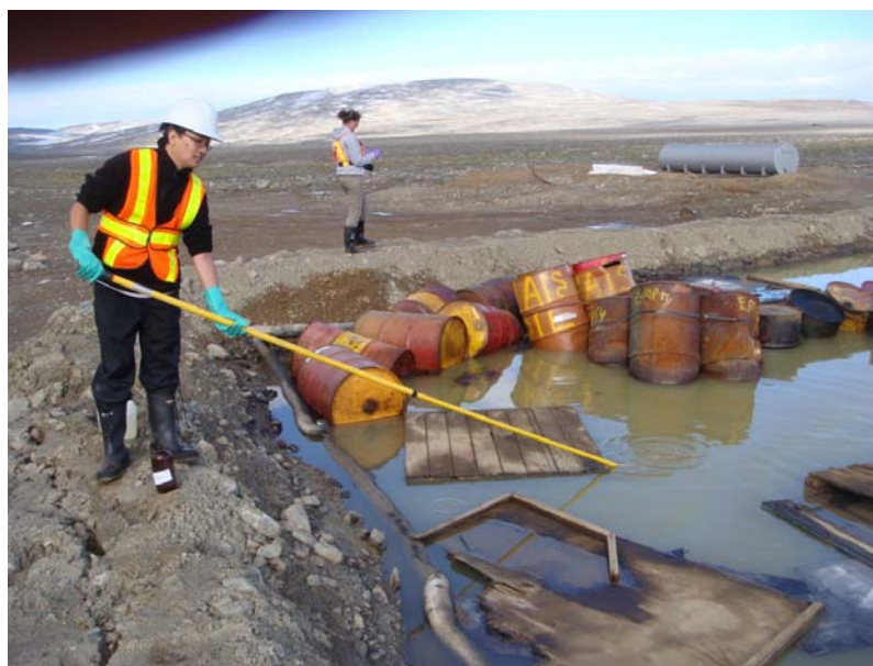
Photo 4 (DSC01466) Sample 10-21299 Dye-M Collecting a composite sample of ponded water from LS BPA - South side
