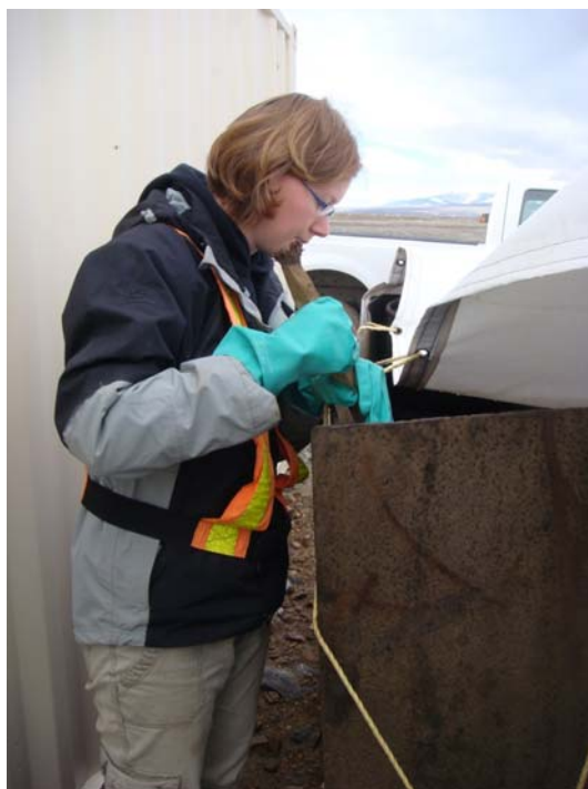
Photo 1 (DSC01722) Sample 10-21336 Dye –M Collecting a sample from a metal container containing wastewater at the tank-farm.
