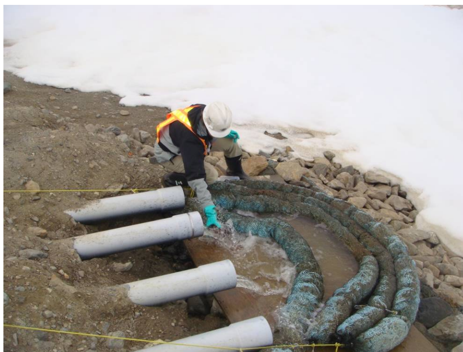
Photo 4 (DSC01014): Sample 10-21244 Dye-M Collecting a wastewater sample from the outflow pipes at the landfarm
