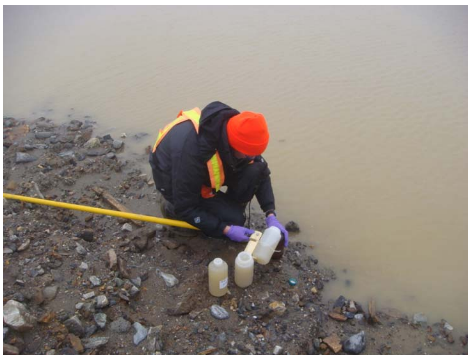
Photo 10 (DSC01670) Sample 10-21327 Dye-M Collecting a sample from the LS NHWL - water pooled in the North east side of the new cell.
