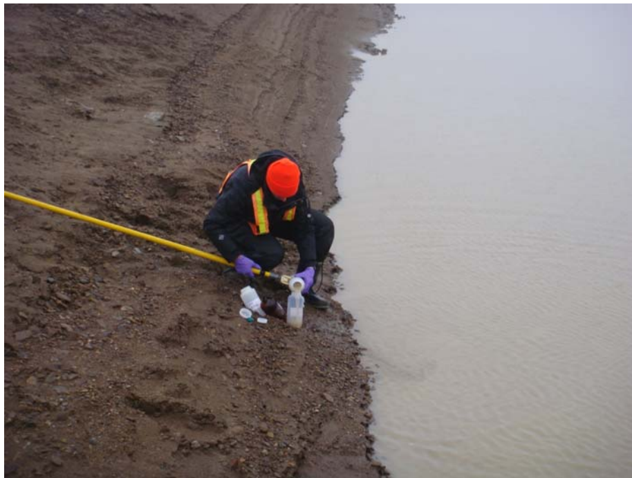
Photo 9 (DSC01646) Sample 10-21326 Dye-M Collecting a sample from pooled water in the LS Tier II - Water pooled all along the north berm
