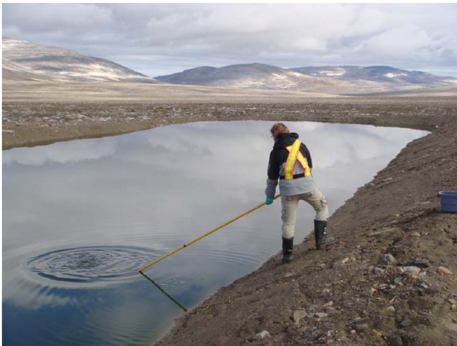
Photo 1 (DSC17525) Sample 10-21328 Dye-M Collecting a sample from the new cell of the sewage lagoon.
