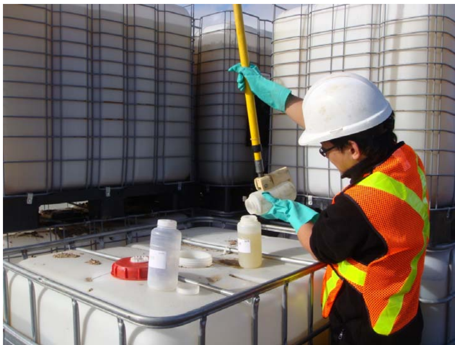
Photo 3 (DSC01464) Sample 10-21298 Dye-M Collecting a sample from a tote in LS BPA (full of ponded water from LS PBA)
