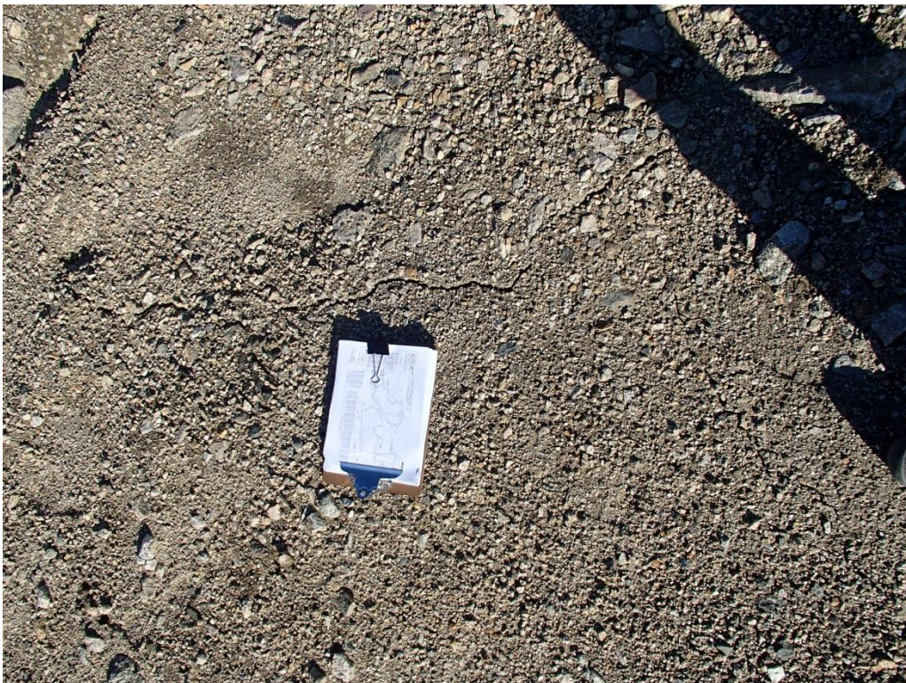
Photograph 70. Minor tension cracks at Lobes 2, 3 and 4 ↑
