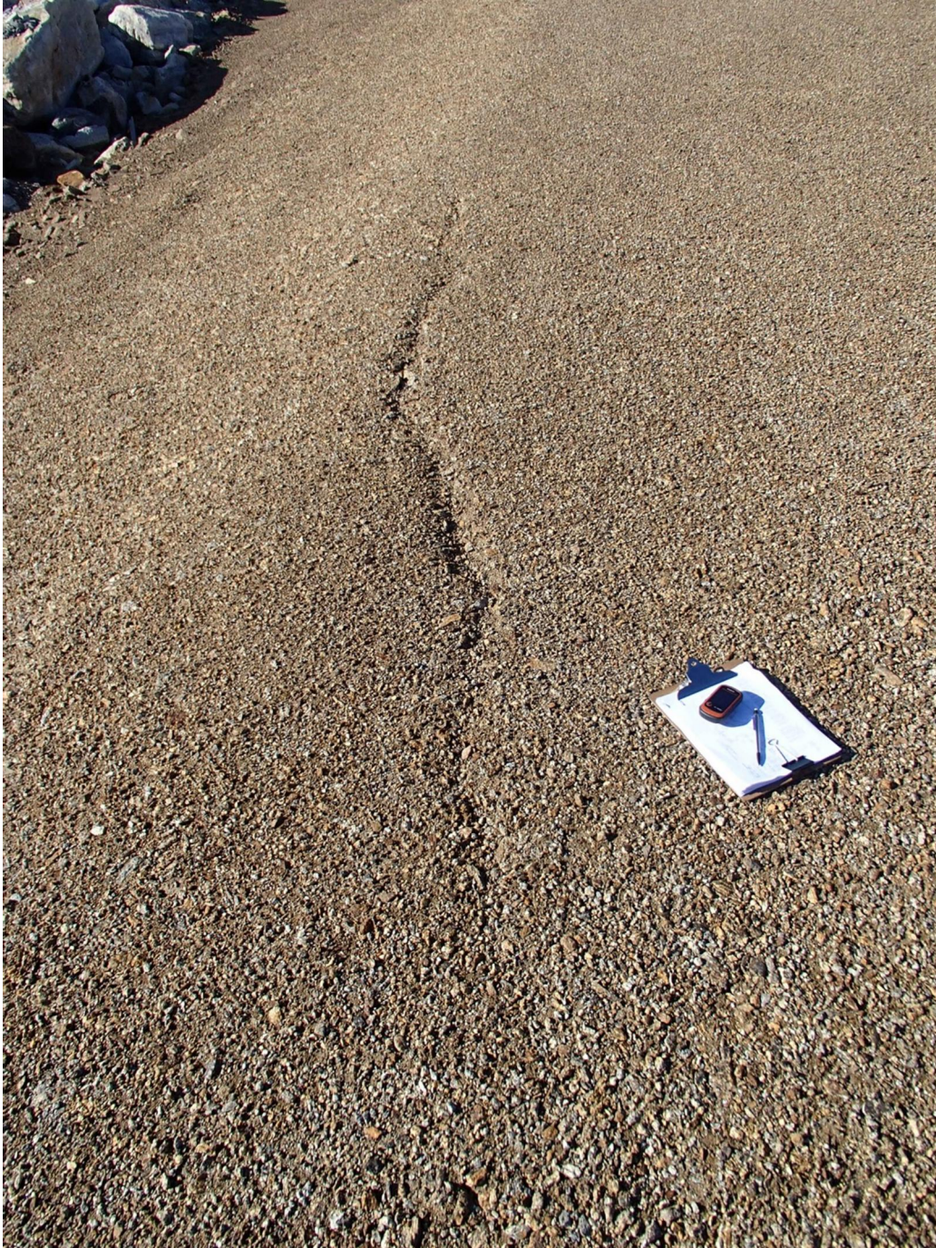
Photograph 80. Minor tension cracks on Lobe 1 ↑
