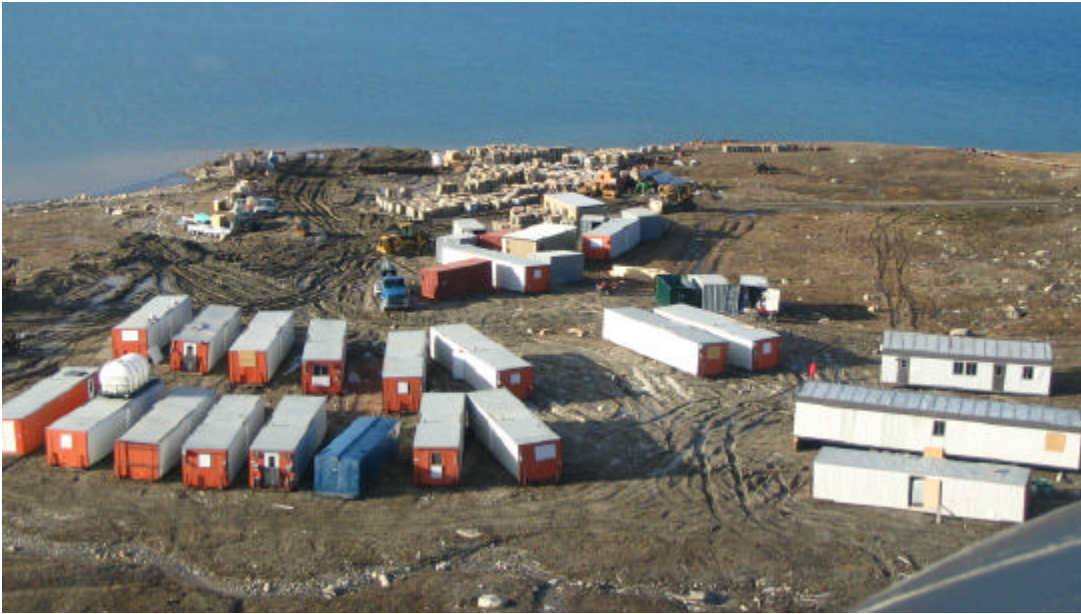
Photo 1: Aerial view of unloaded equipment. Note vehicle rutting resulting from extremely soft soil conditions leading from the beach.
