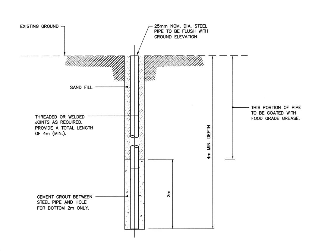
MINIMUM EMBEDMENT CAN BE REDUCED IF ROCK IS ENCOUNTERED. INSTALLATION TO PENETRATE A MINIMUM OF 2m INTO ROCK.
