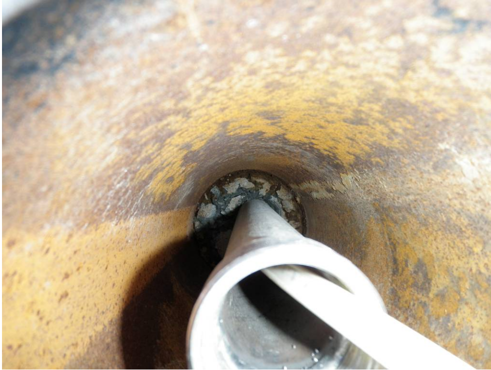
Photo 7. Monitoring well, MW-East, showing a good surface seal with minor cracking. Photograph number P8270371.
