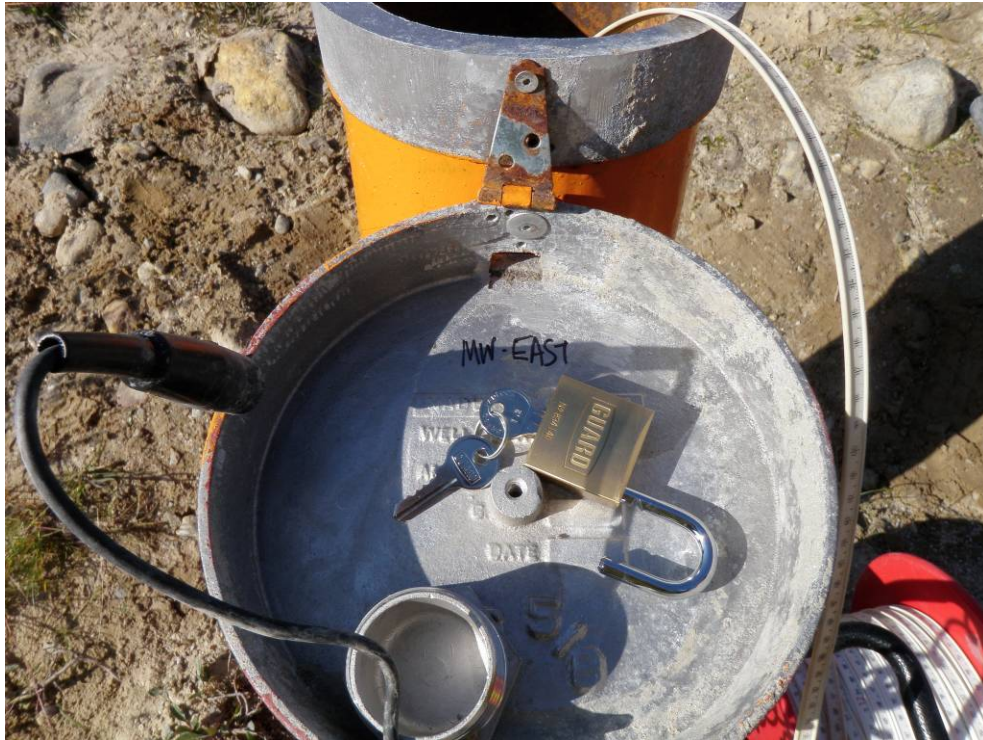
Photo 11. Monitoring well MW-East with failing rivets on lid; rivets have since failed. Photograph number P8270376.
