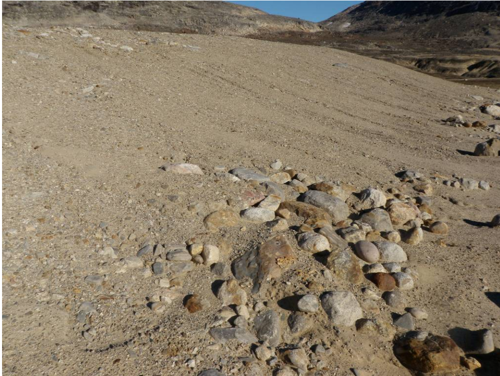
Exposed cobbles at NW corner of landfill at toe of berm. Note the erosion channels in background (Features M & N). Viewpoint 81 (Figure A-1; Appendix A). Photograph reference 81 (CD-ROM). Direction photo taken: S
