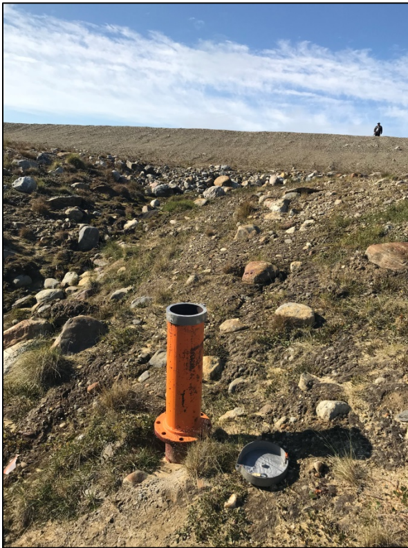
Photograph 9. MW-East showing signs of jacking. Facing west.
