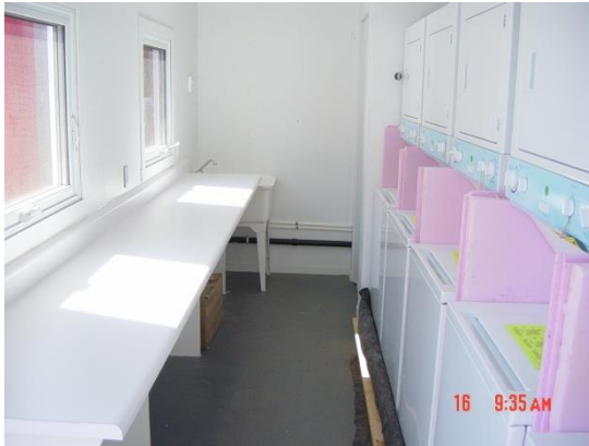
Typical 6 washers/dryers container with: 1 x 2000 watts x 250 cfm ceiling fan heater, 1 x 60 gallons hot water tank, 1 smoke detector and 1 fire extinguisher.
