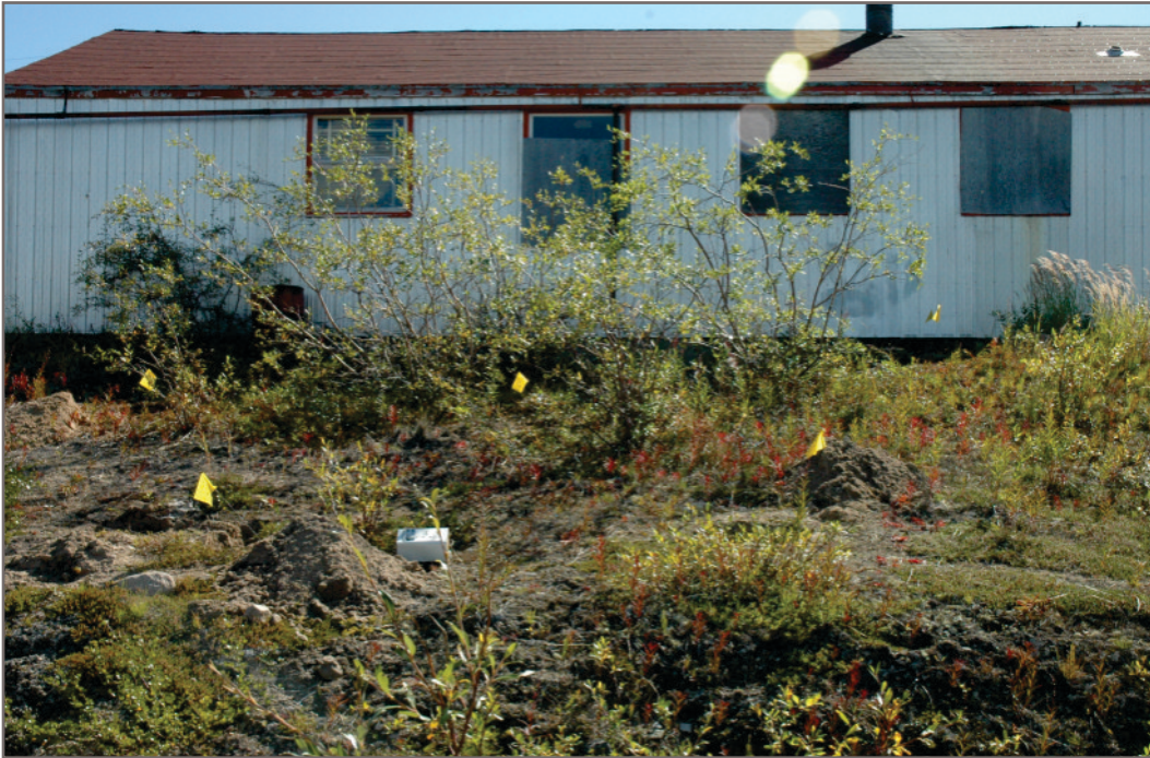
Photo E-15: APEC 13/APEC 14 - Overhead Pipeline/Building 1 - Delineation soil sample locations APEC 13-SS010 to SS017 are shown; hydrocarbon odour was noted at the base of the foundation
