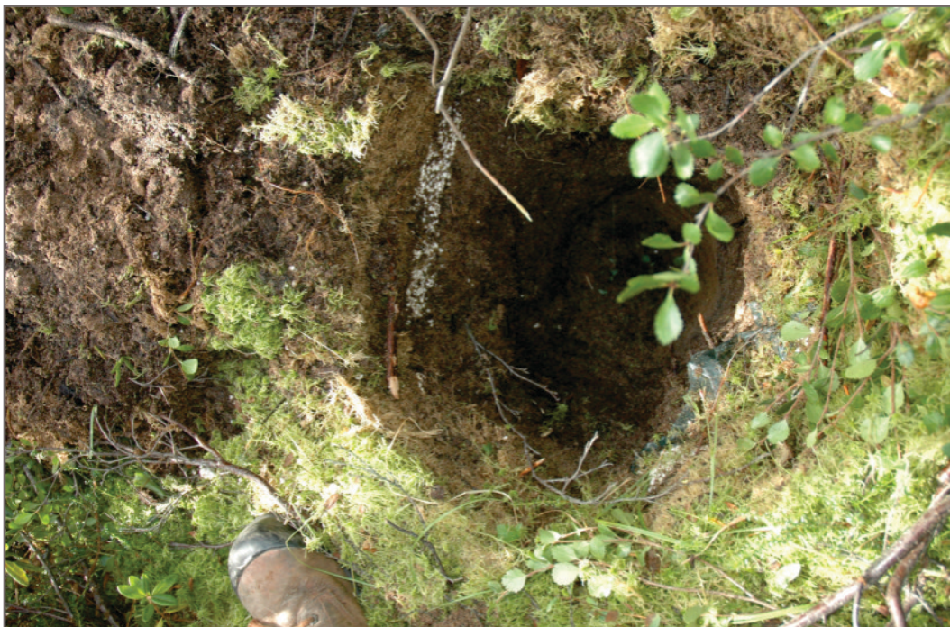
Photo E-10: APEC 8 - Pipeline - Sample location taken down-gradient of APEC1; delineation soil sample APEC 8-SS011 is shown; both samples taken in a low lying depressional area, hydrocarbon odour was noted
