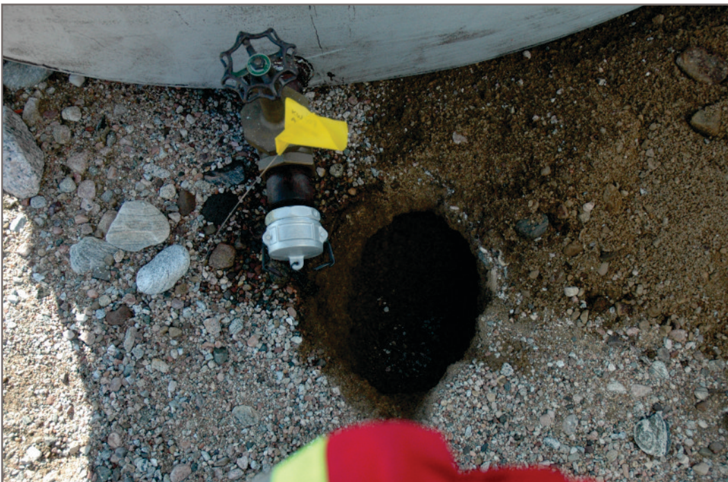
Photo E-8: APEC 4a - Tank 5 - Flag locations for soil samples APEC 4a- SS001, staining was noted at the valve of the AST
