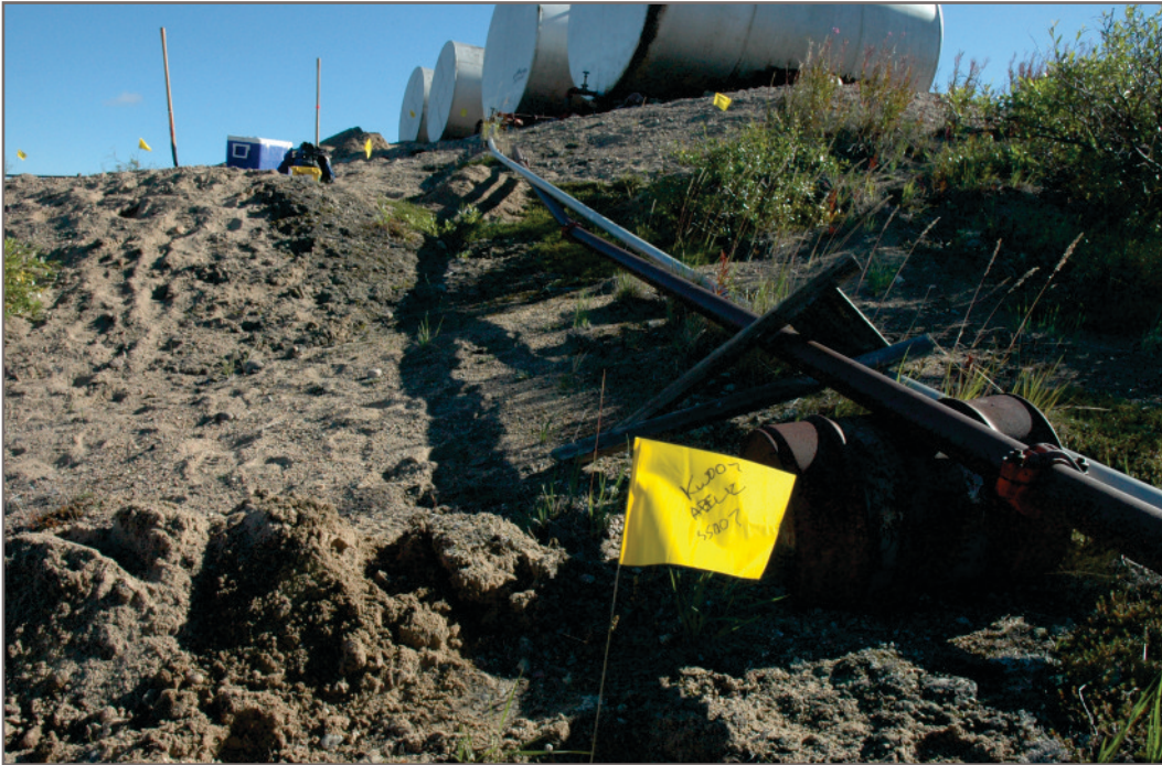
Photo E-13: APEX 12 - Tank 4 - Delineation soil sample APEX 12-SS007 is shown looking north toward the tank farm; in the background soil samples APEX 12-SS001 to SS005 can be seen delineating the hydrocarbon plume
