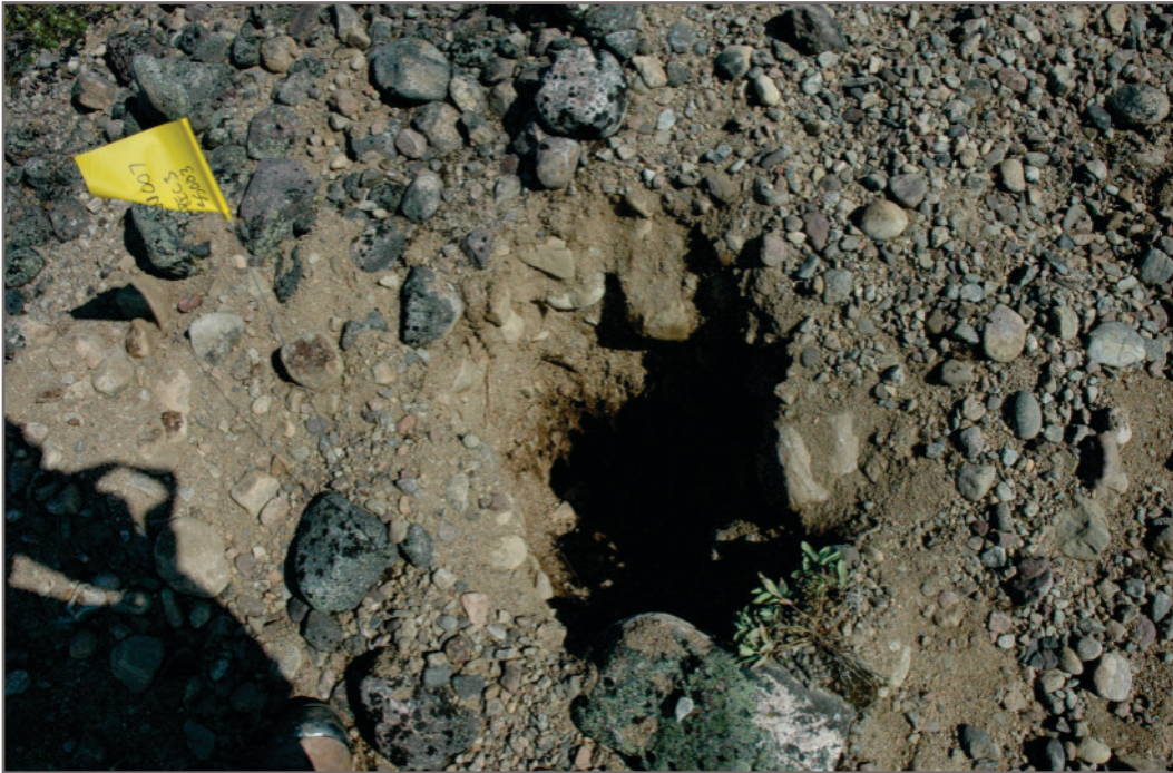
Photo E-29: General Soil Condition at APEC 3 - Sand with an estimated 10 - 20 % cobbles and gravel at terminal extent of pipeline near Stain 3
