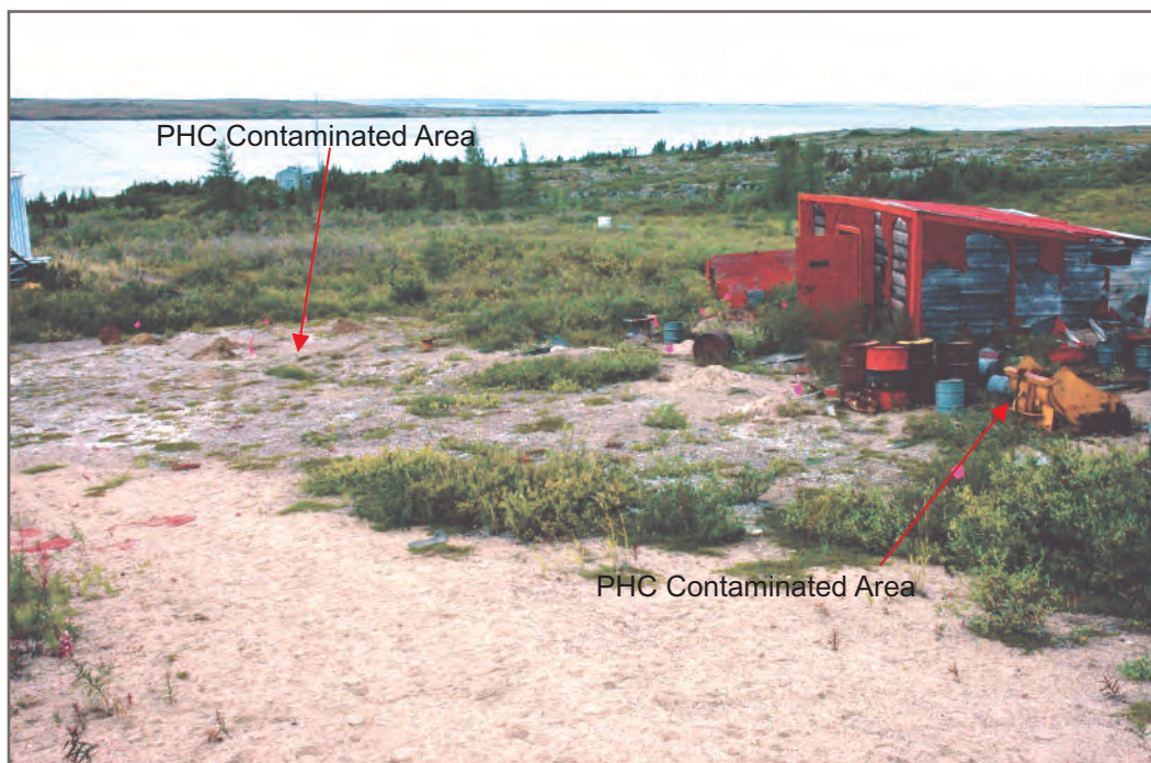
Photo E-22: APEC 19 and 20 - Buildings 7 and 8 - Two areas of hydrocarbon contamination were identified. The approximate locations of the areas are shown.
