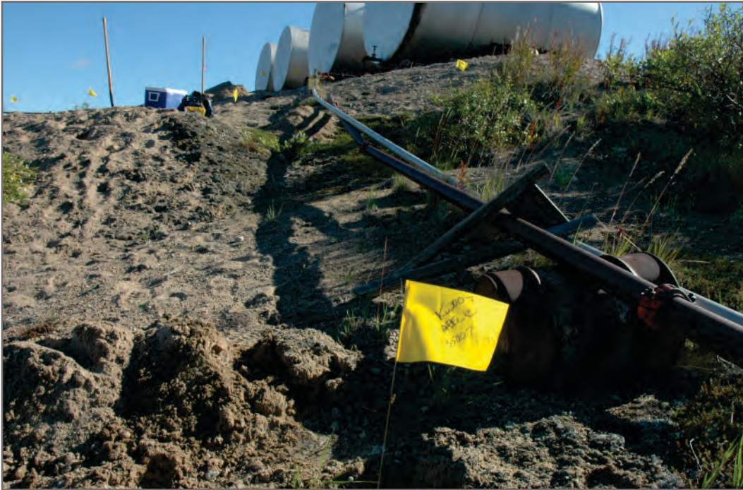
Photo E-13: APEC 12 - Tank 4 - Delineation soil sample APEC 12-SS007 is shown looking north toward the tank farm; in the background soil samples APEC 12-SS001 to SS005 can be seen delineating the hydrocarbon plume
