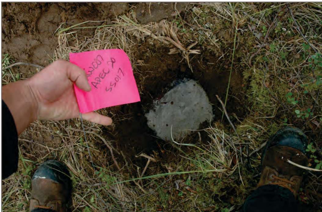
Photo E-24: APEC 20 - Building 8 - Soil sample APEC 20-SS017 is shown; water was encountered upon the completion of the test pit
