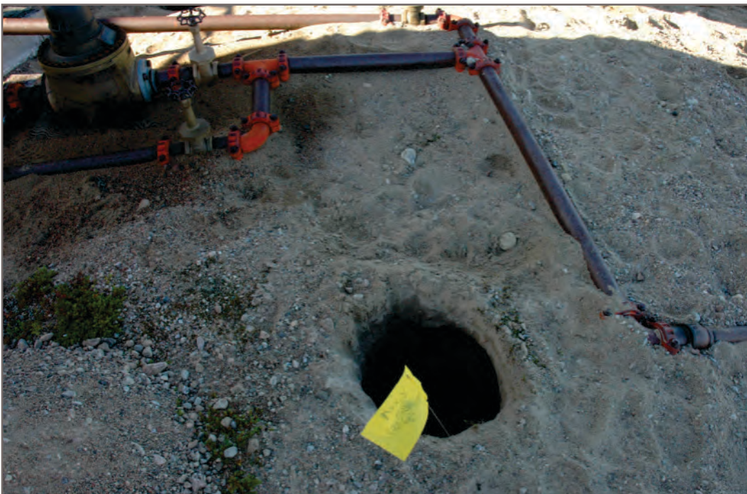
Photo E-12: APEC 9 - Tank 1- Soil sample location APEC 9- SS001; the soil sample was taken down-gradient of the fuel distribution lines; significant hydrocarbon odour and staining around the valves was noted
