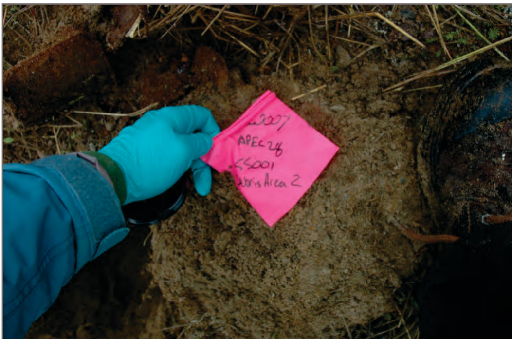
Photo E-26: APEC 28 - Debris Area, organic soil/matter was encountered overlaying sand, multiple layers of waste were discovered during test pitting
