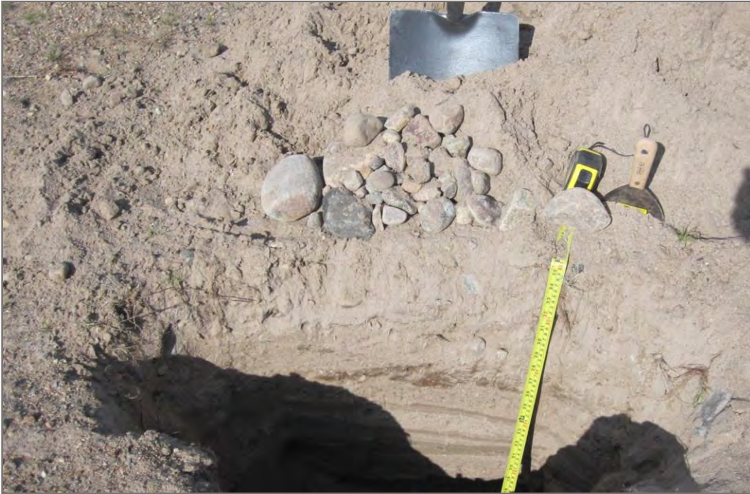
Photo G35: Potential Landfill 2 - Testpit (TP04), showing subrounded gravel removed from testpit.
