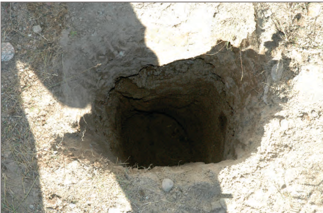
Photo E-30: General Soil Condition at APEC 13 (Central Buildings) - Well sorted sand with some gravel
