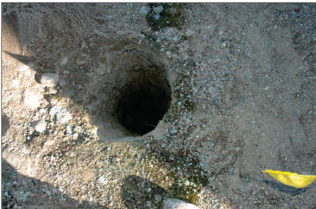
Photo E-28: General Soil Condition taken at APEC 12 - Sand with an estimated 5 - 10% cobbles, located at the toe of APEC 12
