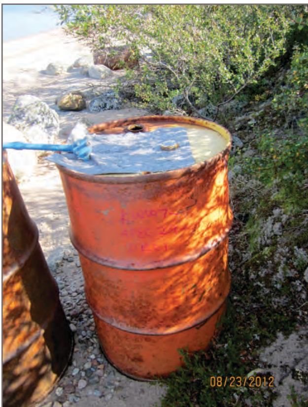
Photo H-59: APEC 29 - Total lead and leachable lead painted drum with blue, flammable content
