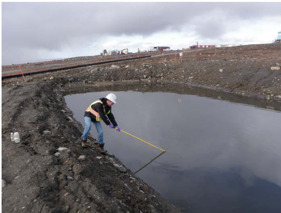
Photo 1 (P9090001) Sample 10-36522 Fox-3: Collecting a sample from the cell 3 of the camp sewage lagoon.
