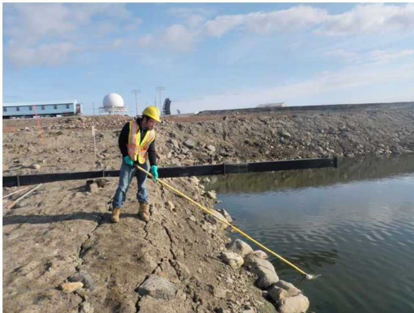
Photo 1 (10-02738) Sewage Lagoon Cell 4 Fox-3: Collecting a sample from Camp Sewage Lagoon – Cell #4.
