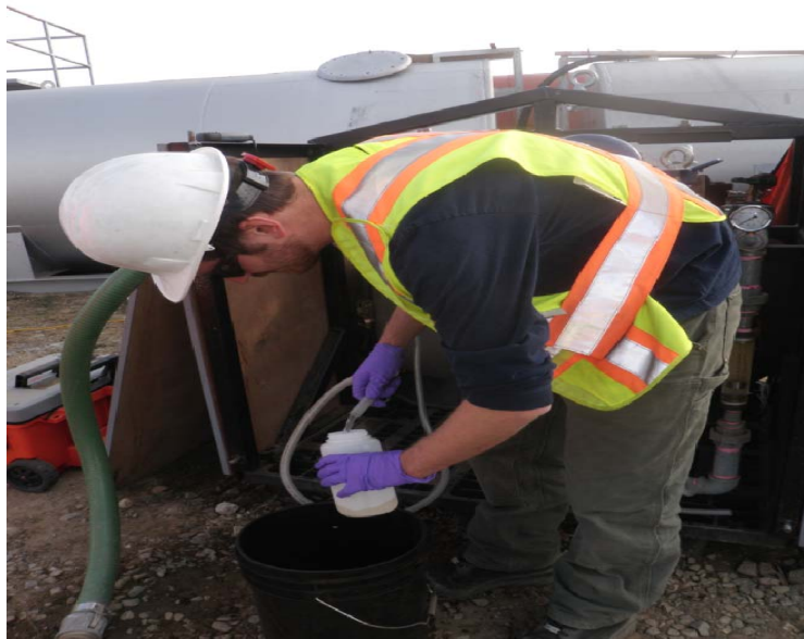
Photo 1 Sample (10-02737) Fox-3: Wastewater Sampling at Contractor Intake Hose.
