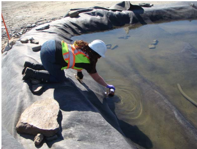
Photo 1 DSC02005 Sample 10-00008 Fox-3: Collecting a sample from the water pooled in the station west fuel storage berm
