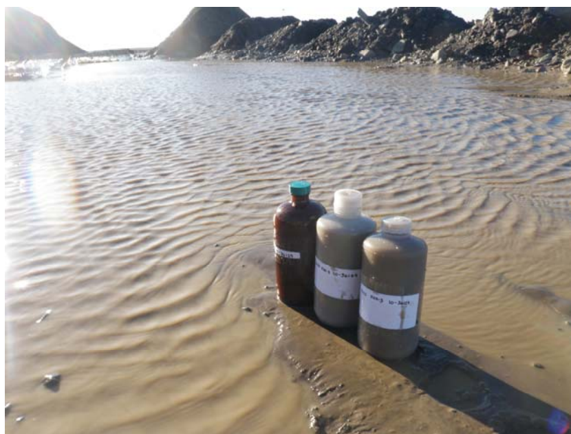
Photo 2 – Sample 10-36129 Fox-3: Wastewater Samples 36129 in amber, Teflon and HDPE bottles, MPA#7.
