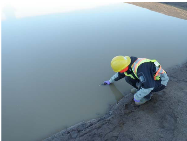
Photo 4 (P9040052) Sample 10-36163 Fox-3: Wastewater sampling at Tier II Facility.
