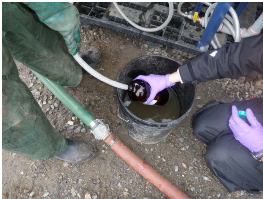
Photo 2 Sample (10-04002) Fox-3: Wastewater Sampling at Contractor Intake Hose
