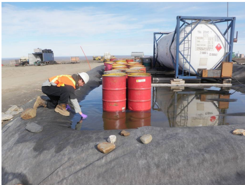
Photo 14 Sample 11-28764 FOX-3: Wastewater sample collected from the Station West Fuel Berm (facing northwest).
