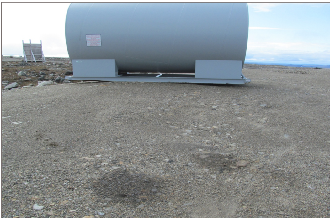
PHOTO 7 IMG 0113: Station West Landfill - Hydrocarbon stains at north end of Lobe A end of landfill.
