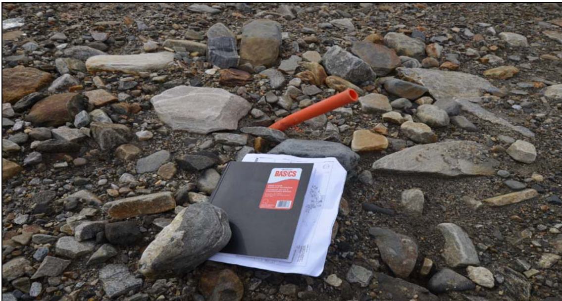
Figure 2: Photo - 2013-F3-SW-13 - Feature C - Close-up - orange plastic pipe in north landfill toe, used to mark material lift heights by surveyors; 1 of 2 plastic pipes present on the Lobe A - (previously observed).
