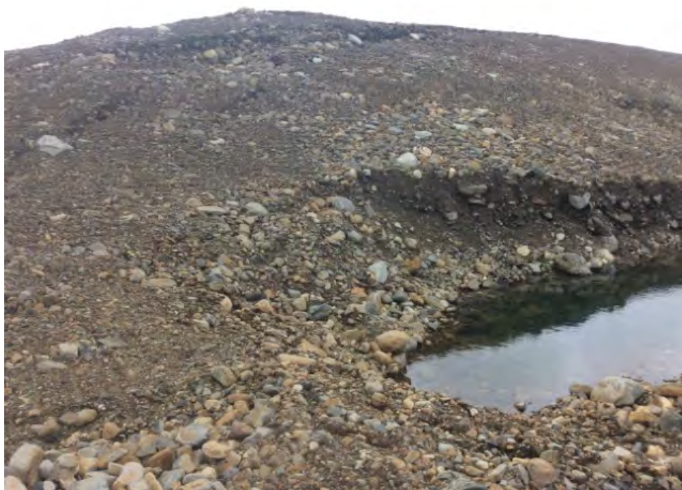
Photo E13: Thermokarst – Feature C - ponded water in low point of thermokarst settlement area (ATT42_Photo1.jpg)
