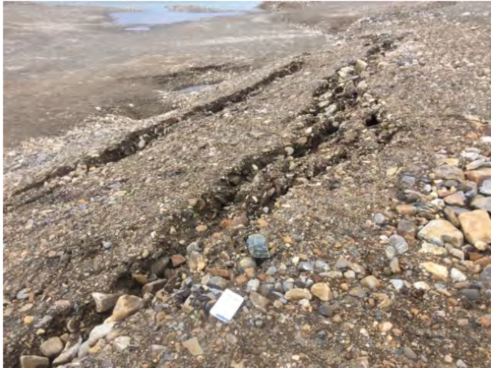
Photo E8: Thermokarst – Top of upper tension crack - Feature B (ATT37_Photo2.jpg)
