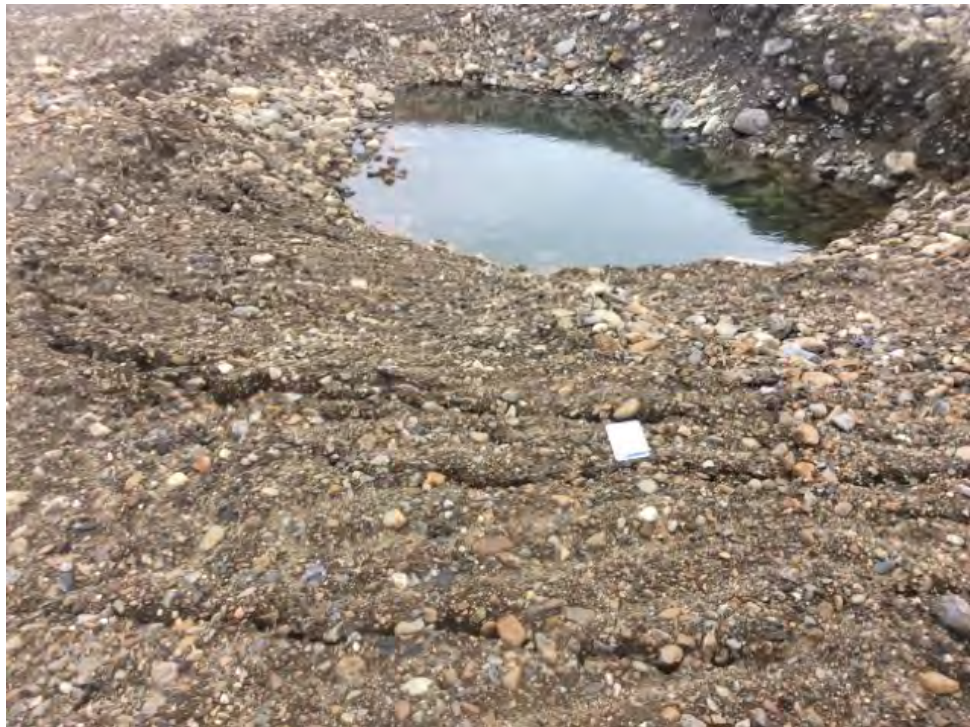
Photo E15: Thermokarst – Feature D - multiple tension cracks towards ponded water in settlement (ATT44_Photo1.jpg)
