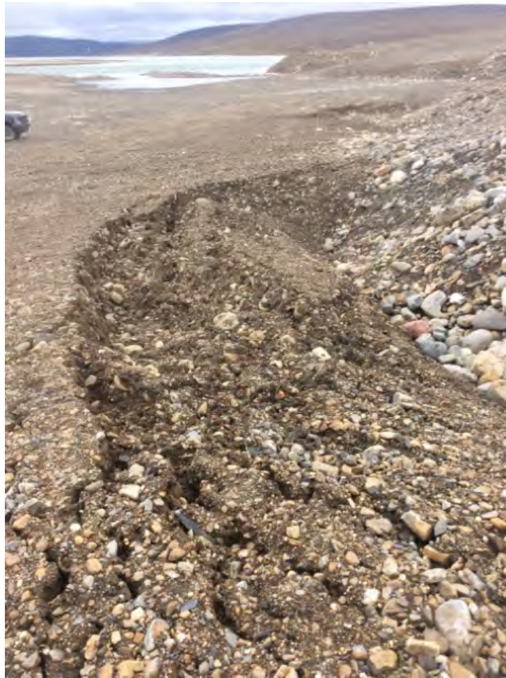
Photo E3: Thermokarst – Perimeter of thaw settlement – Feature A (ATT32_Photo1.jpg)
