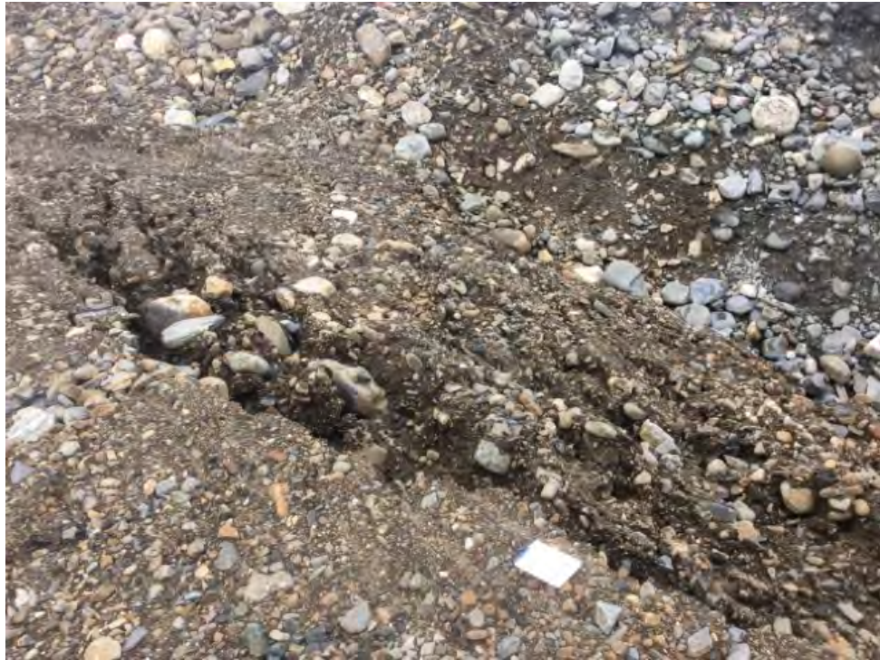
Photo E4: Thermokarst – Feature B - tension crack along thaw settlement perimeter (ATT33_Photo1.jpg)
