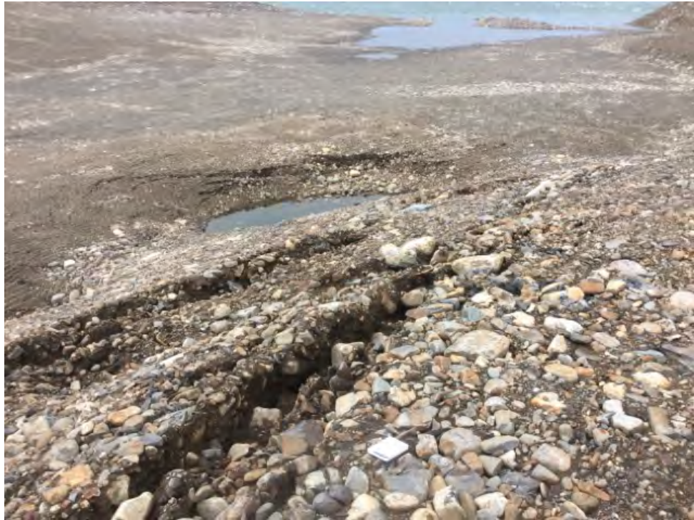
Photo E10: Thermokarst – Top of tension crack - Feature B (ATT39_Photo2.jpg)
