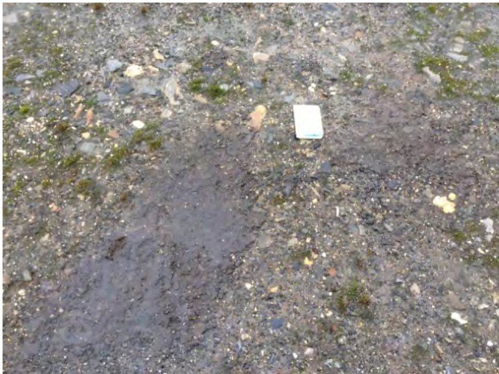
Photo 102: Station West Landfill, Lobe F – Feature N, staining, previously reported as seepage (ATT227_Photo1.jpg)
