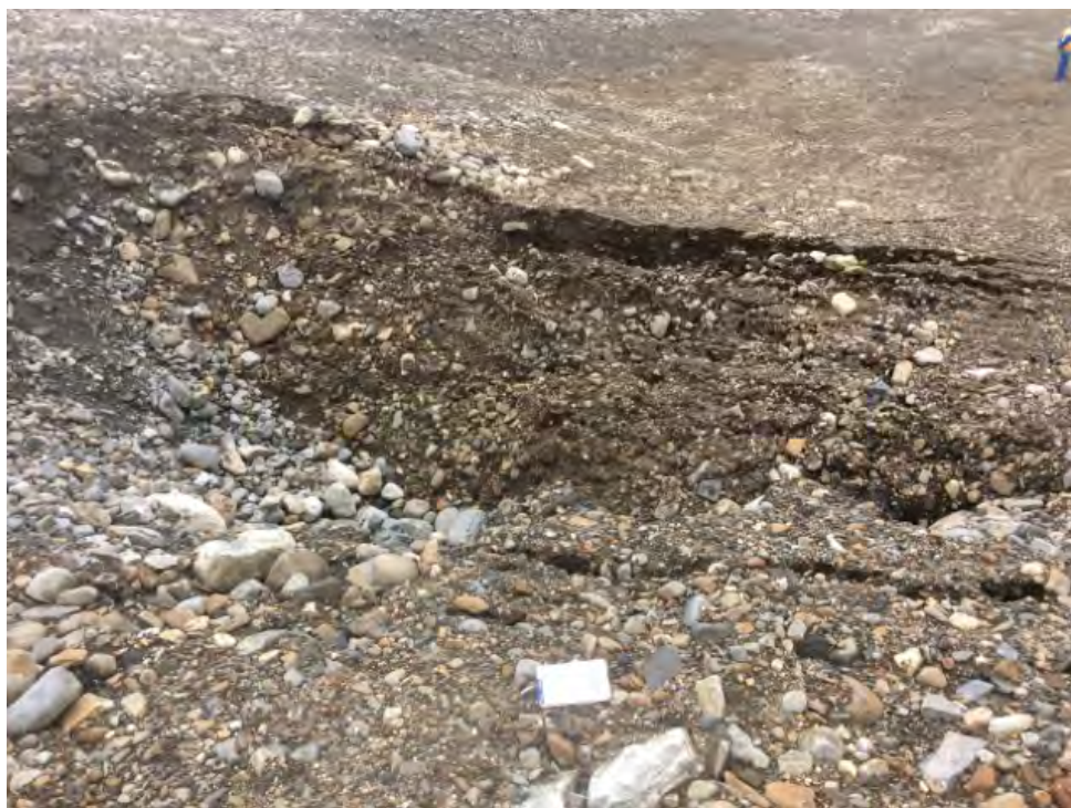
Photo E6: Thermokarst – Feature A - top of thaw settlement slope (ATT35_Photo1.jpg)
