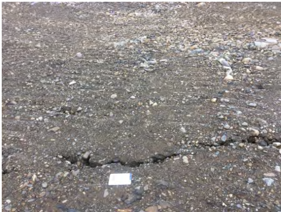
Photo E16: Thermokarst – Tension cracks around settlement area – Facing away from river, 15m long x 0.1m wide (ATT45_Photo1.jpg)
