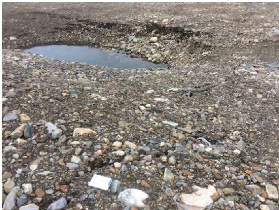
Photo E12: Thermokarst – Top of tension crack (ATT41_Photo2.jpg)
