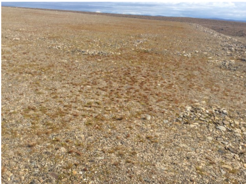
Photo 18: FOX-3 – Non Hazardous Waste Landfill – Cover surface – Feature J – sparse grass vegetation along south crest [Acceptable], facing east (ATT41_Photo41.jpg)
