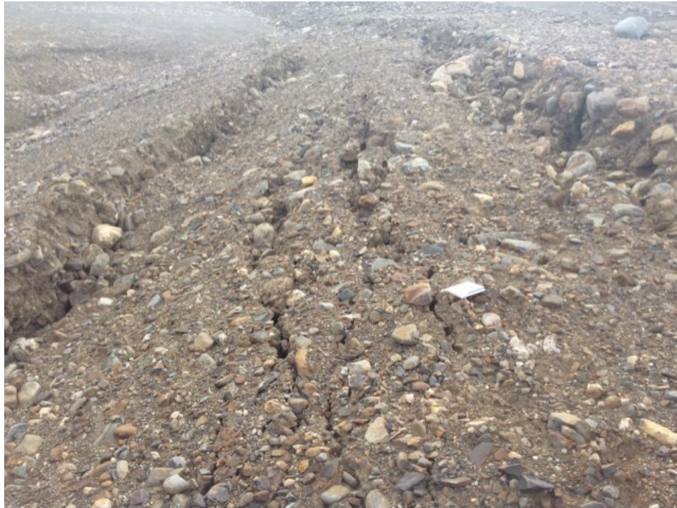
Photo E5: FOX-3 – Thermokarst Area – Feature B – Cracking along the edge of settlement – Looking south (ATT63_Photo63.jpg)
