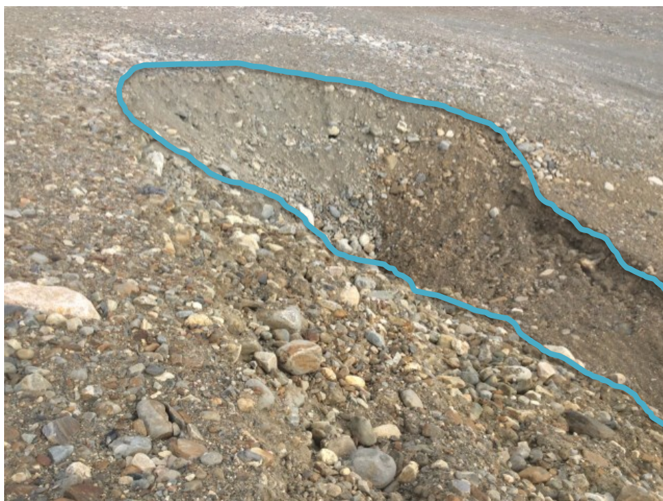
Photo E16: FOX-3 – Thermokarst Area – Settlement area (Feature A), facing northeast (ATT104_Photo104.jpg)
