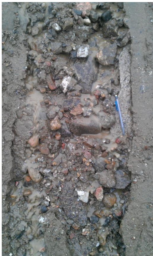
Photograph 44. Helipad West – Self Armouring of Material at Helipad-Landfill West
