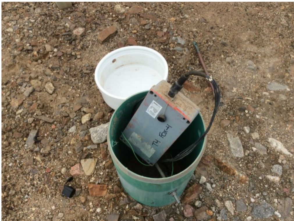
Photo 49: FOX-4 – NHWL/Tier II DF – Thermistor VT-3 (datalogger labeled T4 moved to VT-4) (ATT127_Photo127.jpg)
