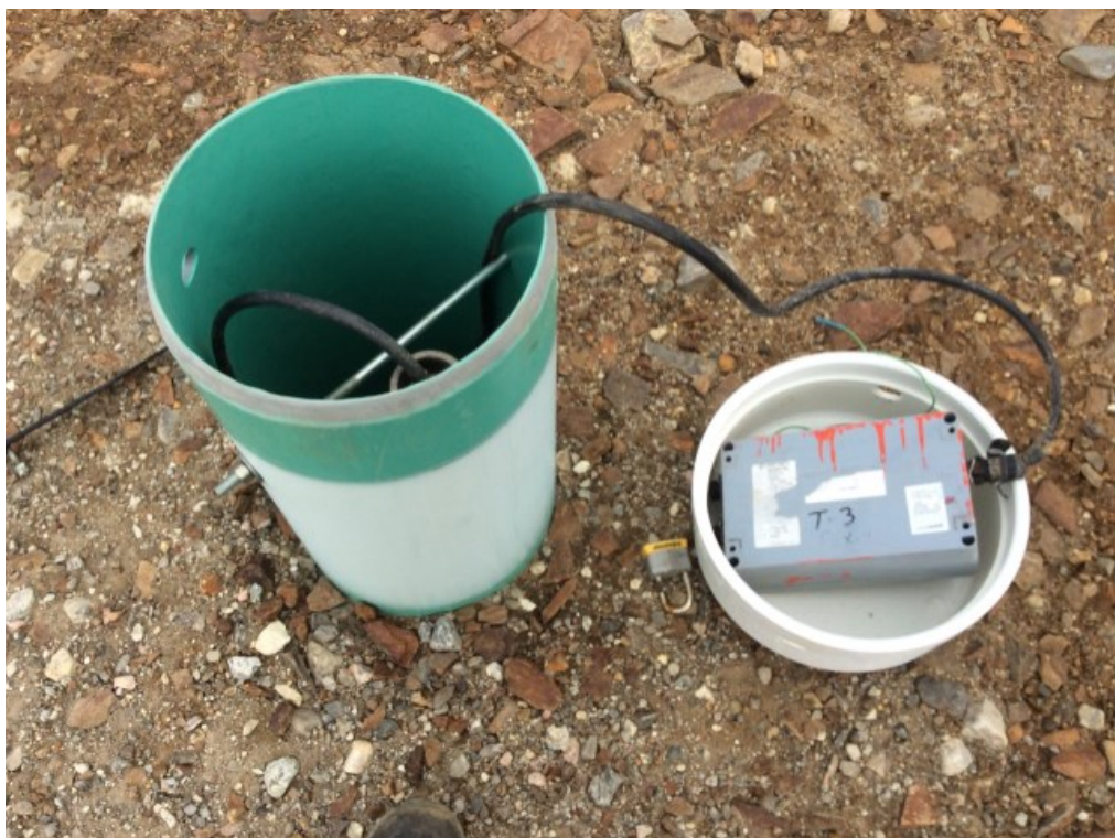
Photo 46: FOX-4 – NHWL/Tier II DF – Thermistor VT-4 (datalogger labeled T3 moved to VT-3) (ATT124_Photo124.jpg)
