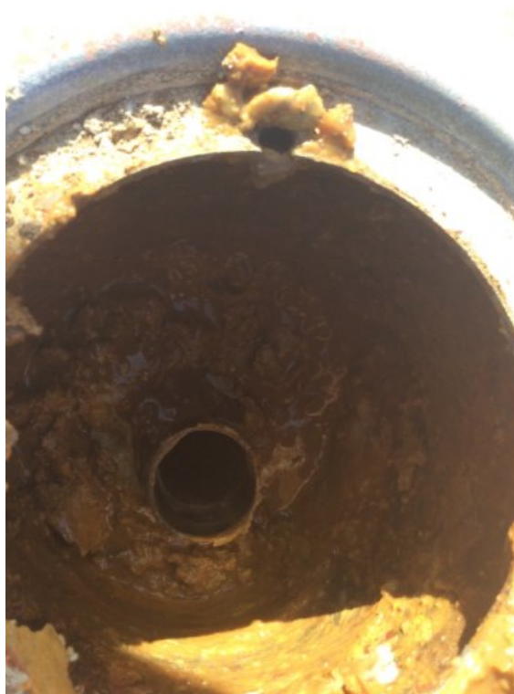
Photo 137: FOX-4 – Station Area Landfill – MW98-07 monitoring well casing filled with bentonite (ATT69_Photo69.jpg)
