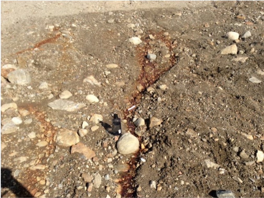
Photo 99: FOX-4 – Helipad West Landfill – Feature J – Orange staining and seepage with sheen, soft saturated ground – West toe facing east (Acceptable) (ATT155_Photo155.jpg)
