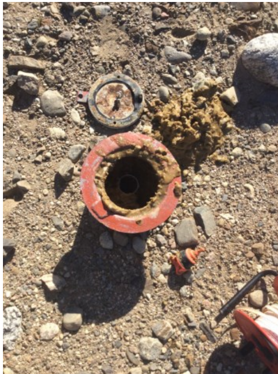
Photo 148: FOX-4 – Station Area Landfill – MW98-09 with bentonite inside protective casing (ATT74_Photo74.jpg)
