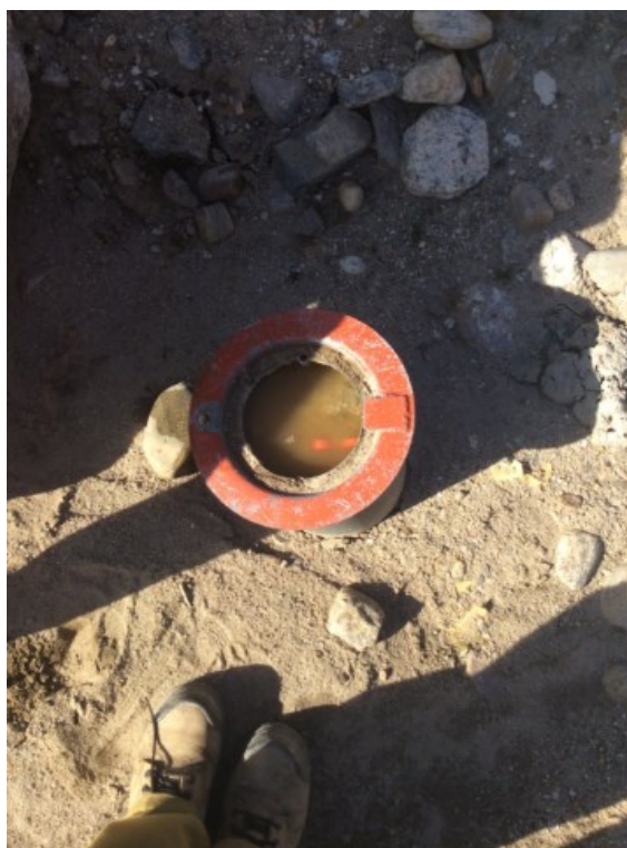
Photo 111: FOX-4 – Helipad West Landfill – MW98-02 monitoring well casing full of water and bentonite (ATT79_Photo79.jpg)
