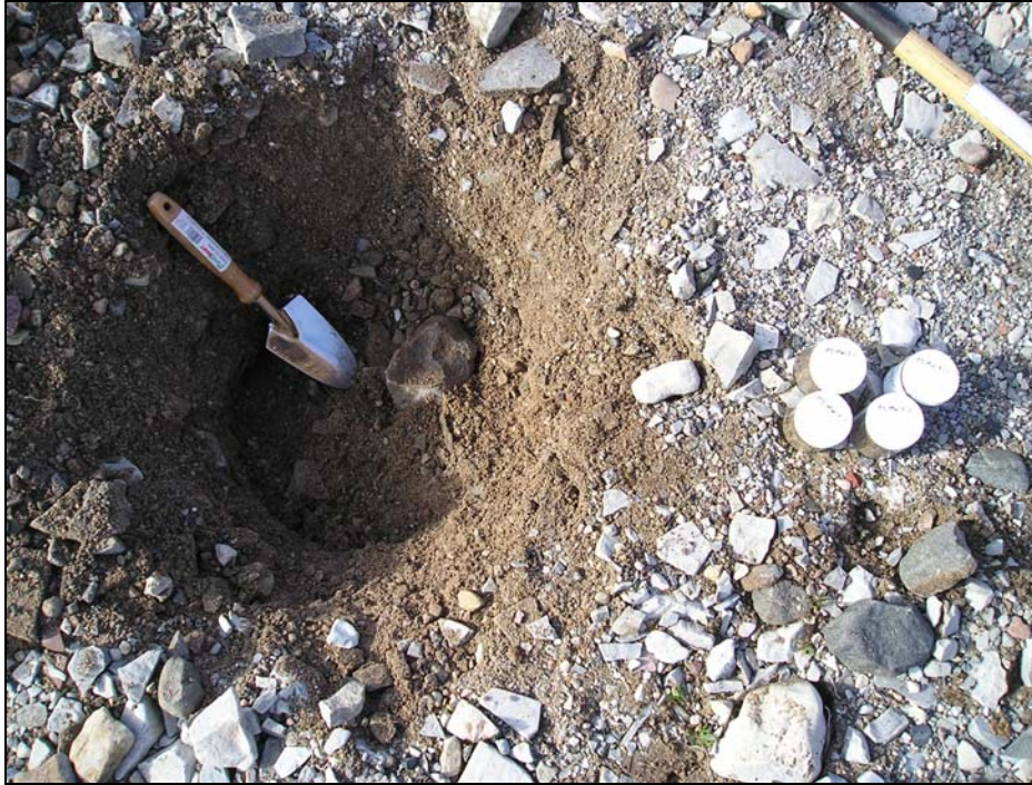
Photograph 3. Test Pit P3-MW-7. Samples P3-MW-7-1 and P3-MW-7-2 collected. Bedrock reached at ~40cm.↑
