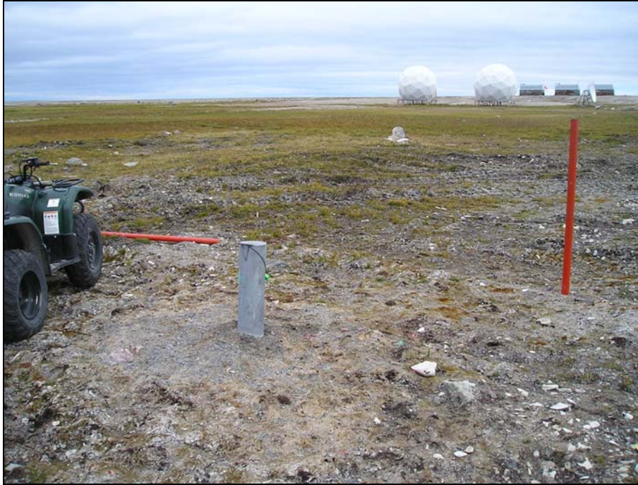
Photograph 3. One of the red markers for MW-14 has fallen over.↑
