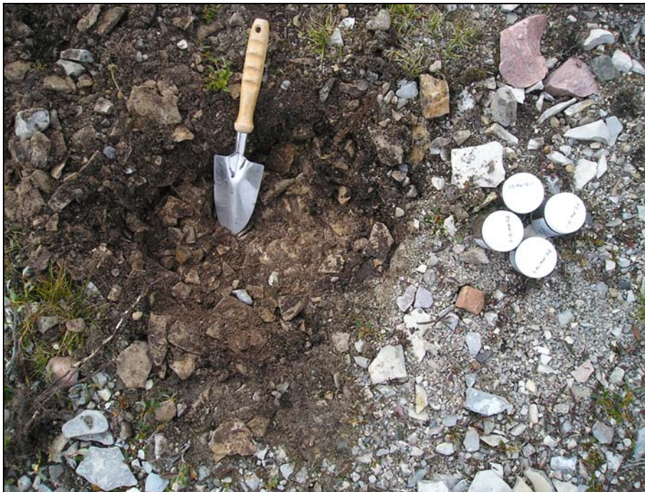
Photograph 4. Test Pit P3-MW-16. Samples P3-MW-16-1 and P3-MW-16-2 collected. Bedrock reached at ~15cm.↑
