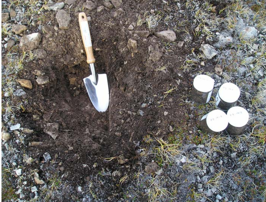
Photograph 3. Test pit P3-14. Samples P3-14-1 and P3-14-2 collected. Bedrock reached at ~30cm.↑
