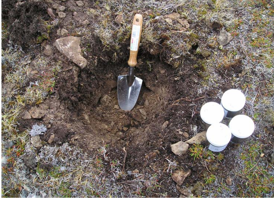
Photograph 1. Test pit P3-1. Samples P3-1-1 and P3-1-2 collected. Bedrock reached at ~40cm.↑
