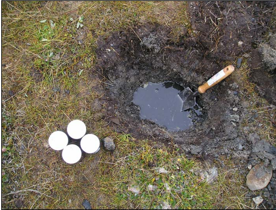
Photograph 7. Test pit P3-11. Samples P3-11-1 and P3-11-2 collected. Water table reached at ~30cm.↑
