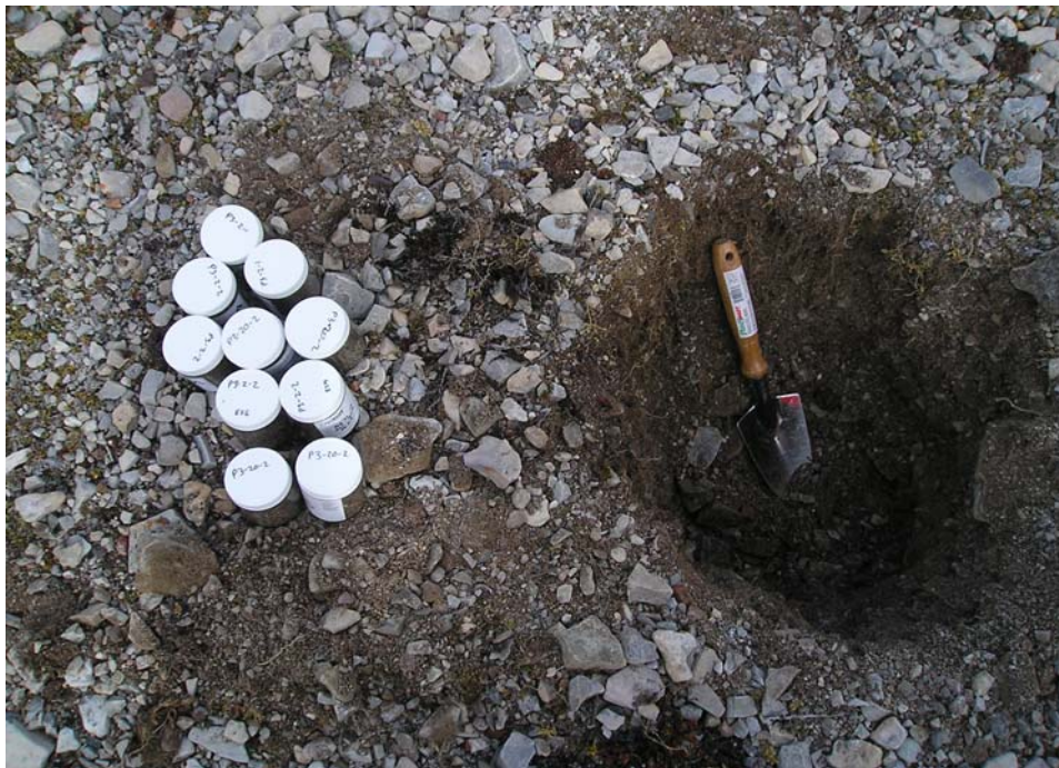
Photograph 2. Test pit P3-2. Samples P3-2-1, P3-2-2, and P3-20-2 (Duplicate of P3-2-2) collected.↑
