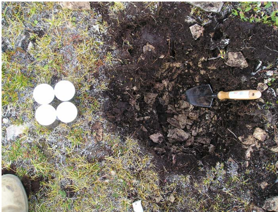
Photograph 4. Test pit P3-4. Samples P3-4-1 and P3-4-2 collected. Bedrock reached at ~40cm.↑
