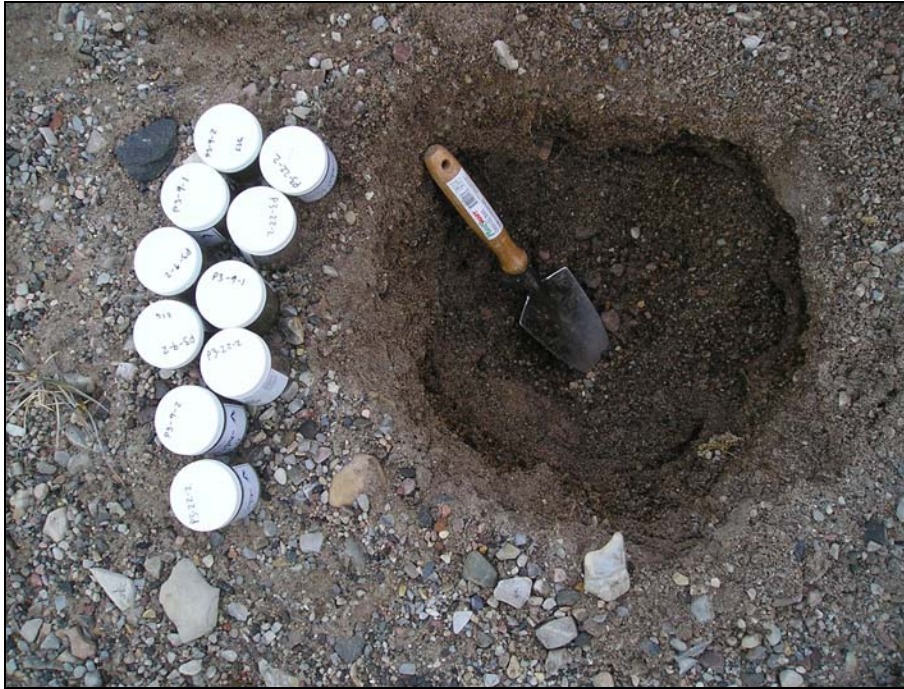
Photograph 5. Test pit P3-9. Samples P3-9-1, P3-9-2, and P3-22-2 (Duplicate of P3-9-2) collected.↑
