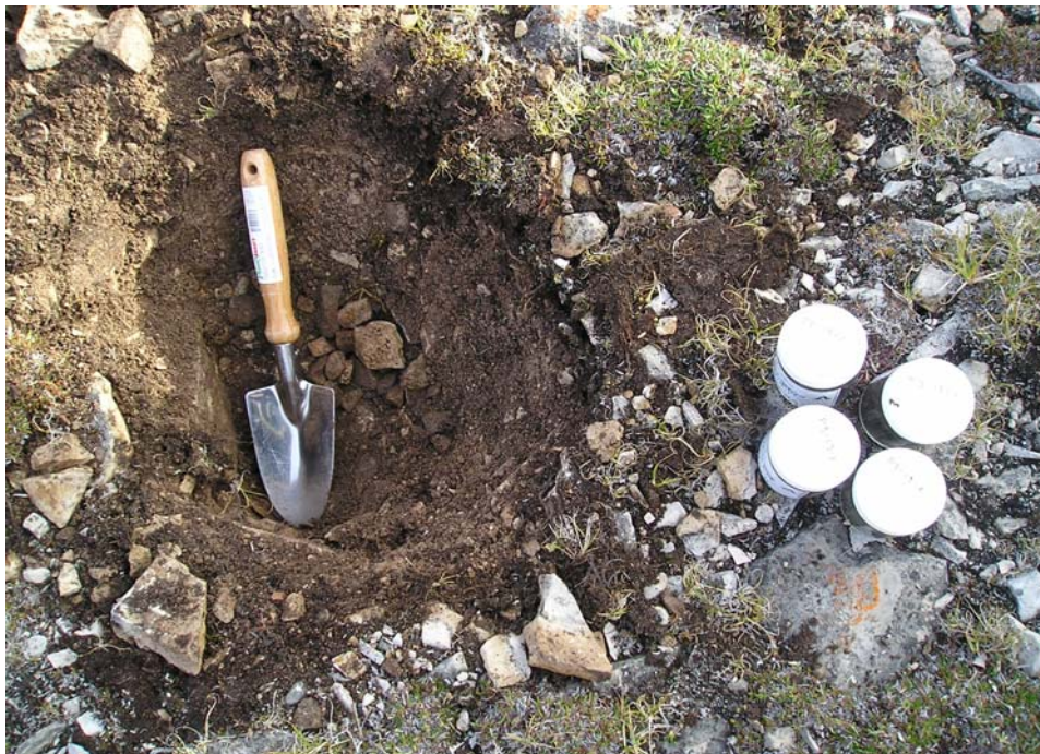
Photograph 2. Test pit P3-13. Samples P3-13-1 and P3-13-2 collected. Bedrock reached at ~40cm.↑
