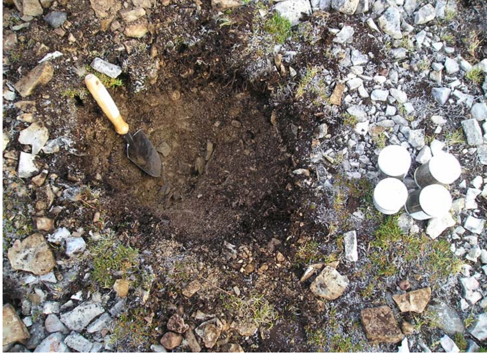
Photograph 1. Test pit P3-12. Samples P3-12-1 and P3-12-2 collected. Bedrock reached at ~40cm.↑
