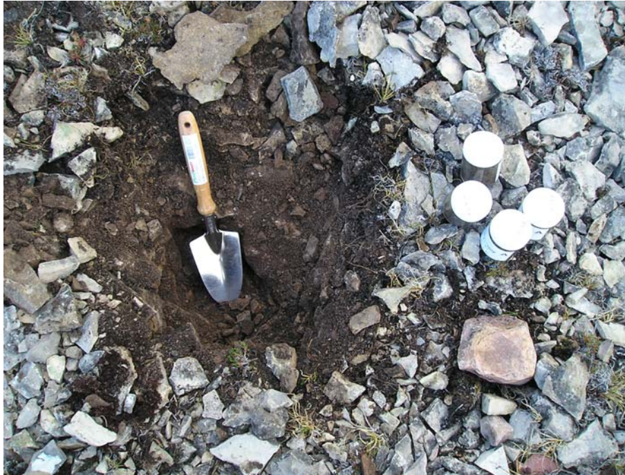
Photograph 5. Test pit P3-16. Samples P3-16-1 and P3-16-2 collected. Bedrock reached at ~40cm.↑
