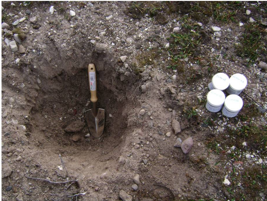
Photograph 4. Test pit at MW-6. Samples P3-MW-6A and P3-MW-6B collected.____ ↑
