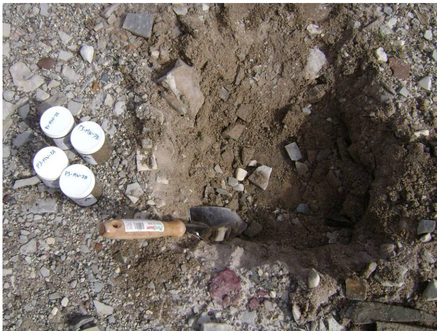
Photograph 6. Test pit at MW-7. Samples P3-MW-7A and P3-MW-7B collected. Bedrock at 0.15m____ ↑
