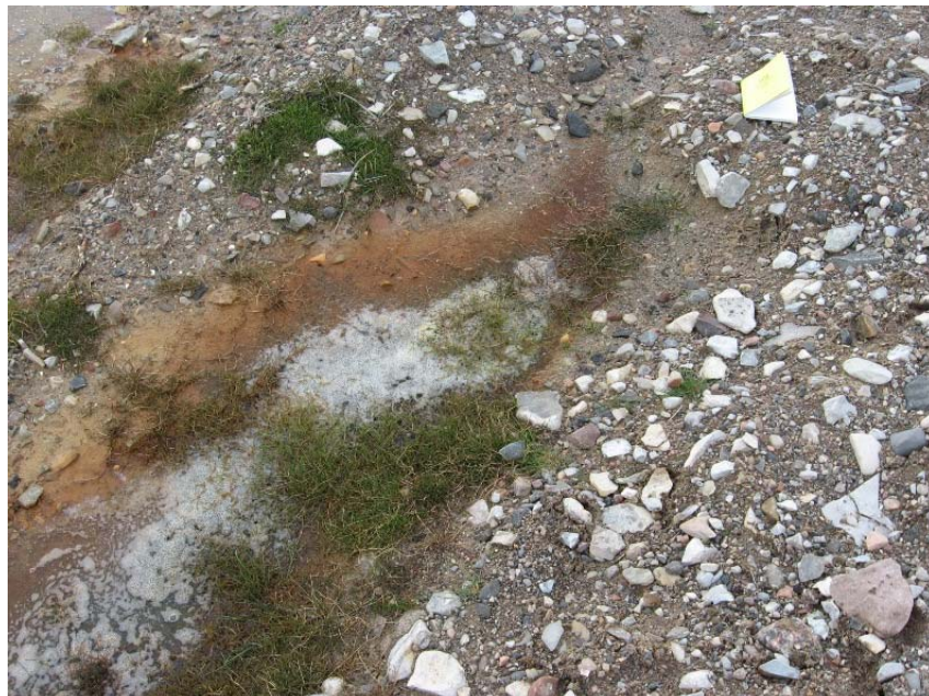
Photograph SLF-16. Close-up of seepage point along the southern perimeter of the East Cell. Same point photographed last 2 years. ↑
