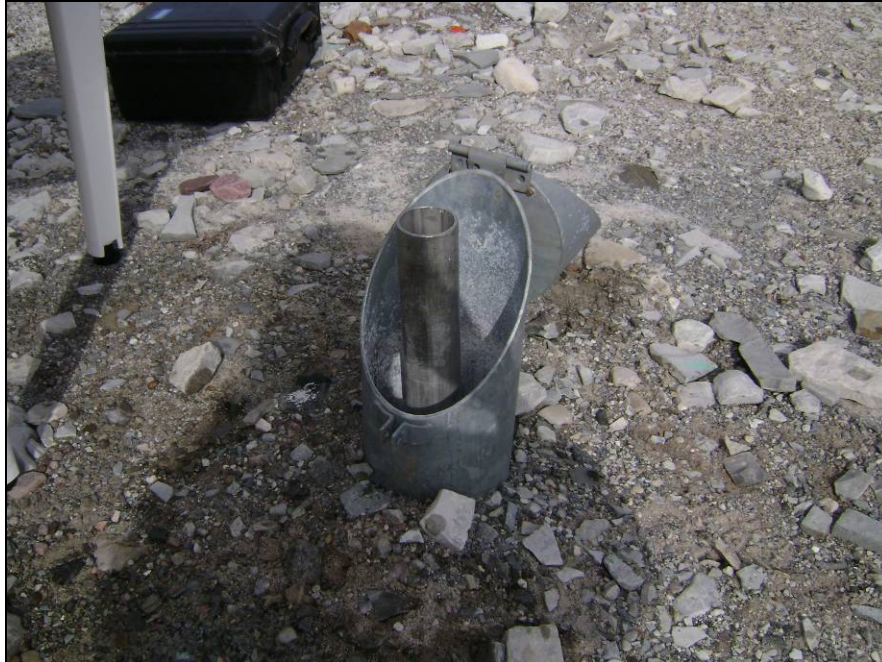
Photograph 5. Monitoring well MW-7. Sample P3-MW-7 collected from flow-through cell. Well ran dry during purge. No appreciable recharge. ↑
