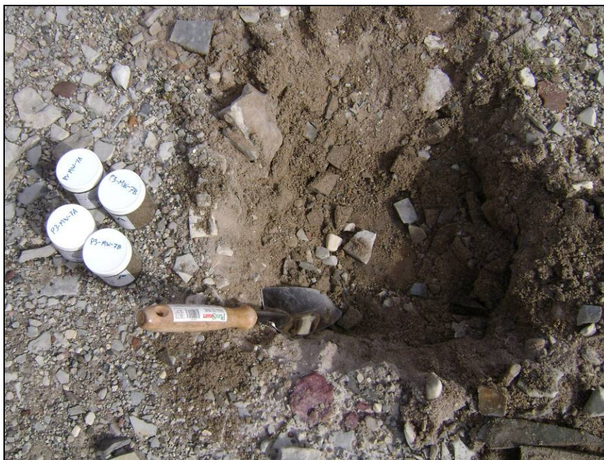
Photograph 6. Test pit at MW-7. Samples P3-MW-7A and P3-MW-7B collected. Bedrock at 0.15m ↑
