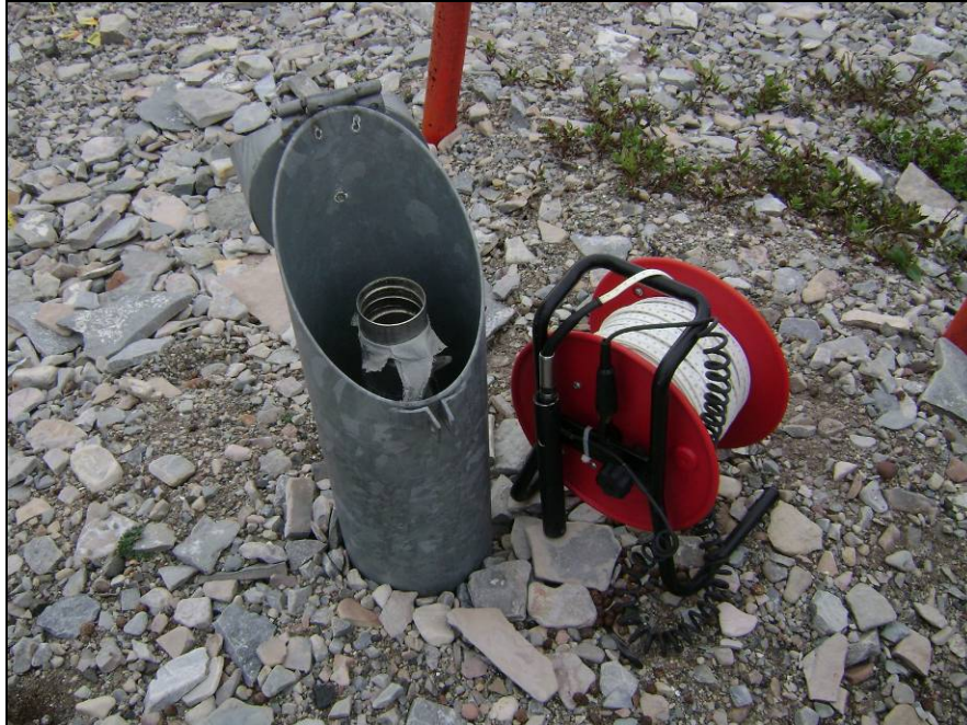
Photograph 1. Monitoring well MW-9. Well frozen at 1.97m. No water for sampling. ↑
