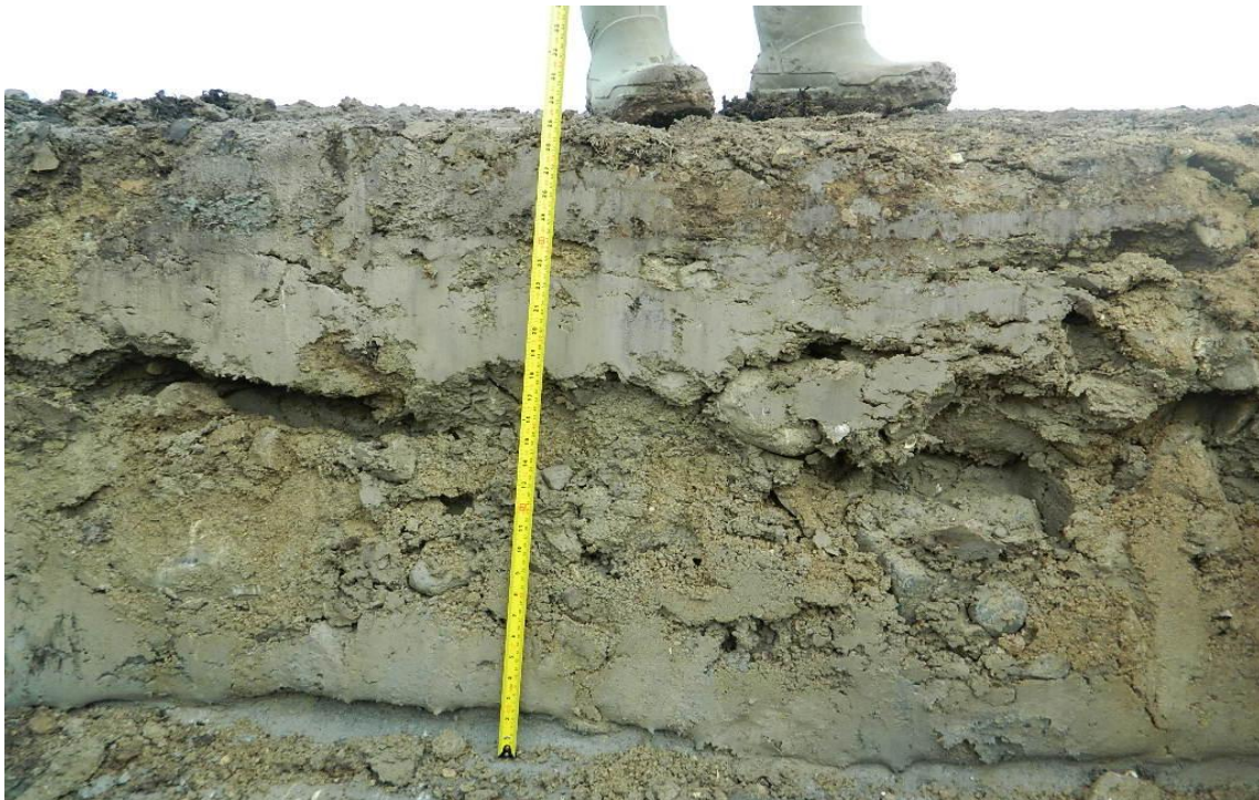
Photo #29: One of four test pits dug to examine soil conditions within FTA LTU.
