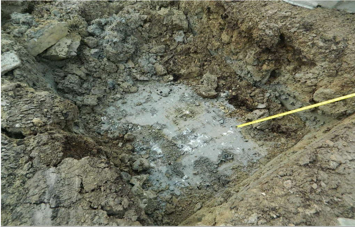
Photo #29: One of four test pits dug to examine soil conditions within FTA LTU.
