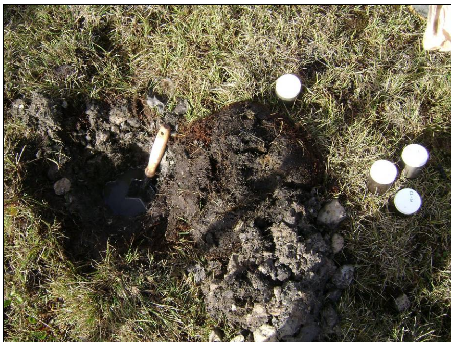
Photograph 2. Test pit at C2-2. Samples C2-2A and C2-2B collected. Water table at 0.20m.↑
