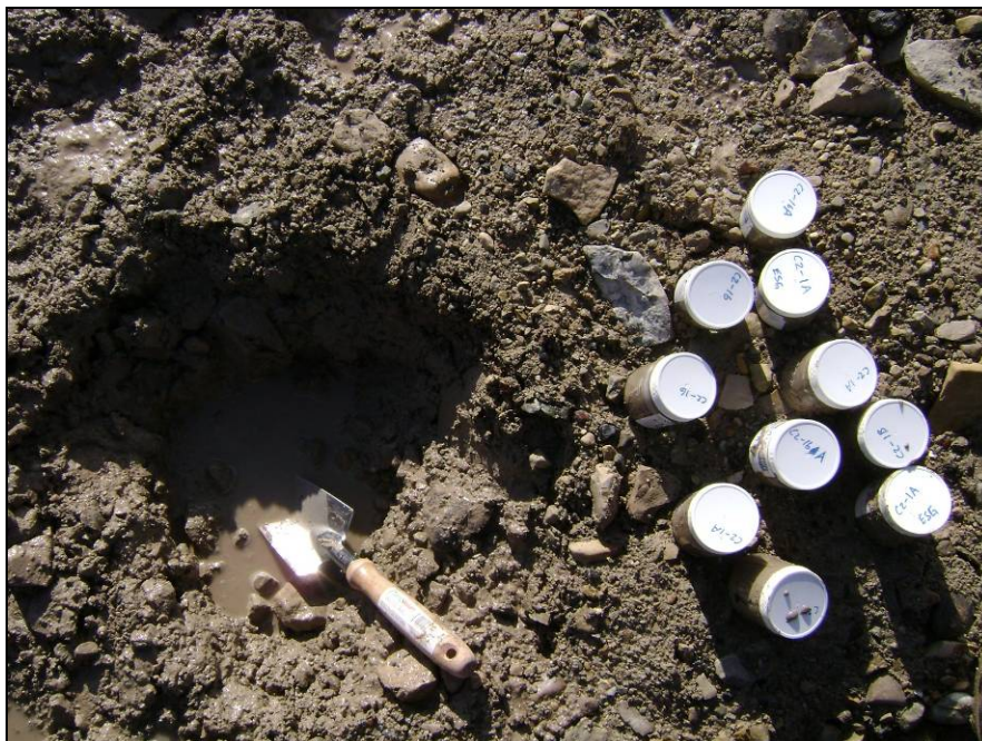
Photograph 1. Test pit at C2-1. Samples C2-1A, C2-1B, and C2-16A (Duplicate) collected. Water table 0.20m.↑
