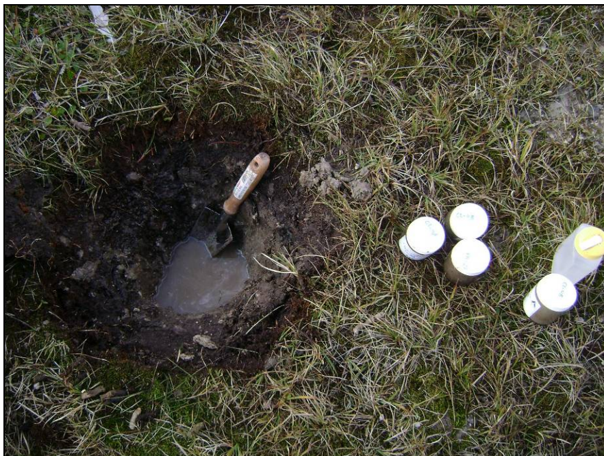
Photograph 4. Test pit at C2-4. Samples C2-4A and C2-4B collected. Water table at 0.10m.↑
