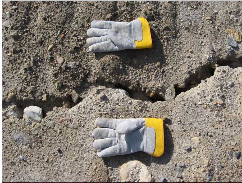
Photograph T2-25. Close-up of old crack noted in T2-24. No indications of recent movement. Slope appears stable. ↑
