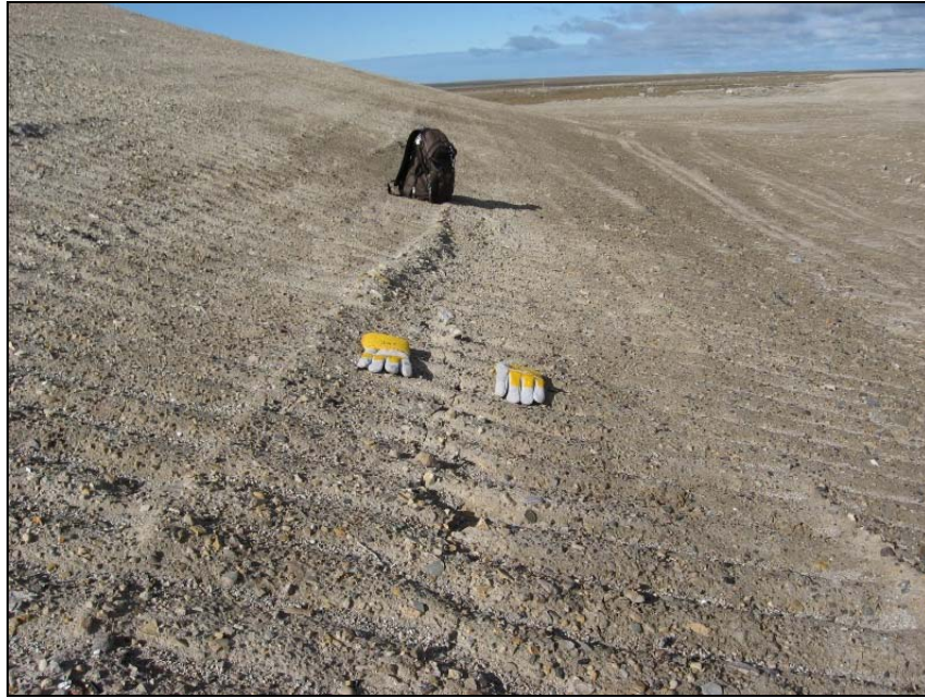
Photograph T2-23. Looking W along N slope to old crack. 1 to 7mm wide, largely eroded/in-filled. Backpack at end (starts 5m E, ends 12m W). ↑
