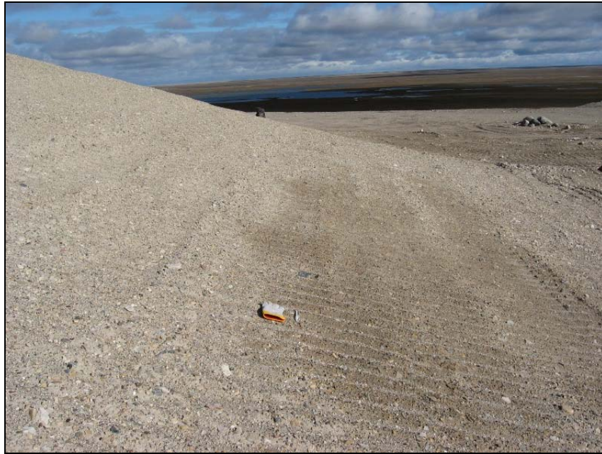
Photograph T2-17. Looking N to NE corner. Fine crack starts between glove and pen and progresses around corner to just downslope of backpack and continues at roughly same elevation for another 35m, splays up to 1 m offset. No indications of recent movement. ↑
