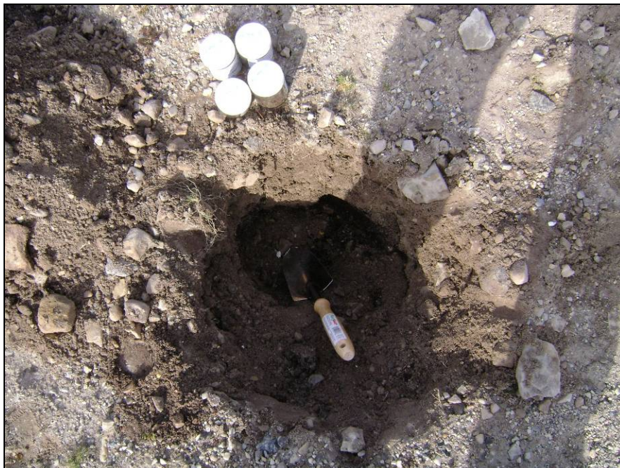
Photograph 2. Test pit at MW-1. Samples C2-MW-1A and C2-MW-1B collected. ↑
