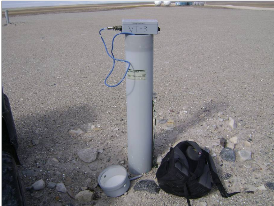
Photograph 11. Vertical thermistor VT-3. ↑
