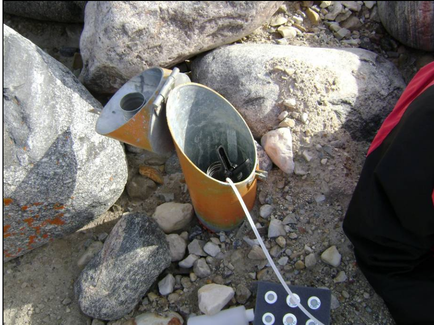
Photograph 3. Monitoring well MW-2. Sample C2-MW-2 collected. ↑
