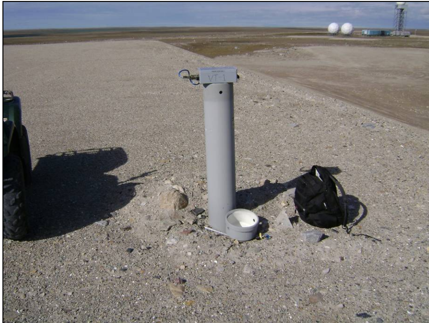
Photograph 9. Vertical thermistor VT-1. ↑
