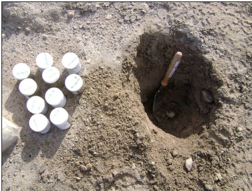
Photograph 4. Test pit at MW-2. Samples C2-MW-2A, C2-MW-2B, and C2-MW-9A (Duplicate) collected. ↑
