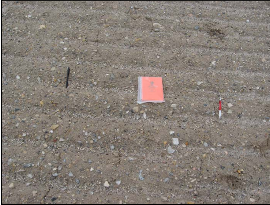
Photograph 21. Following continuation of tension crack noted in Photo 20 (black pen) and noting the start of a second lower crack (red pen). Sediment infilling partially masks cracking. ↑
