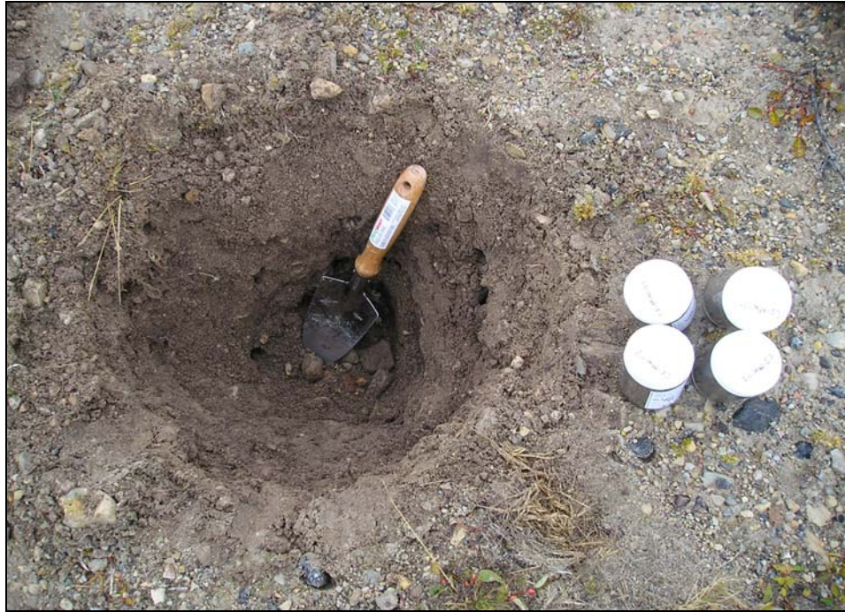
Photograph 1. Test pit C2-MW-1 (Upgradient). Samples C2-MW-1-1 and C2-MW-1-2 collected. ↑
