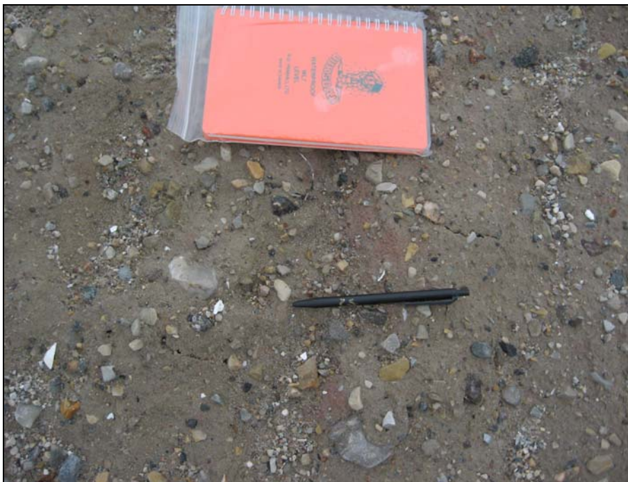
Photograph 22. Possible tension crack (faint and infilled) near top of slope (2m from top). ↑
