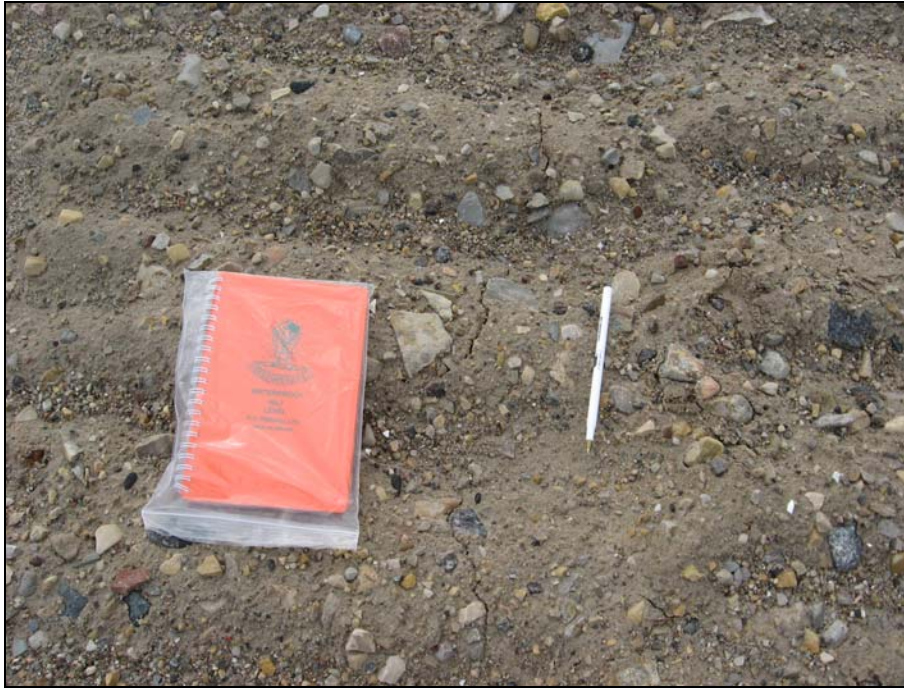
Photograph 9. Following mid-slope tension crack on north face (continues from Photo 8) . Crack splays into minor parallel cracks about 0.5m to 1.0m apart and rejoins. ↑
