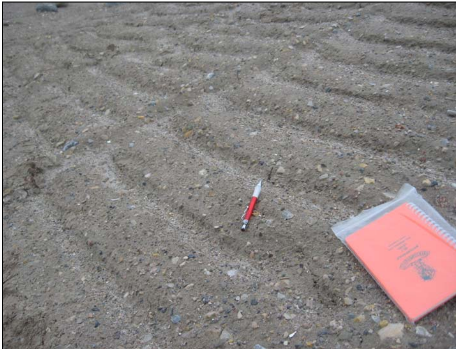
Photograph 30. Tension crack observed in Photo 28 appear to end (likely due to stabilizing influence of downslope granular pad). ↑
