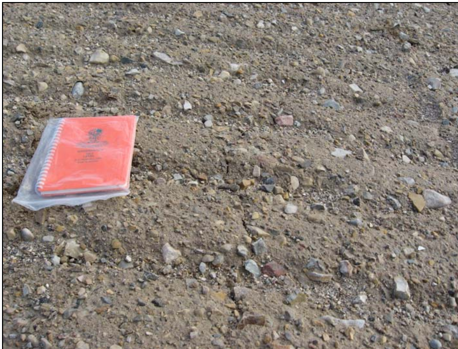
Photograph 14. Tracking the lower tension crack south along the toe of the slope. The tension crack appears to run along the entire toe of slope. ↑
