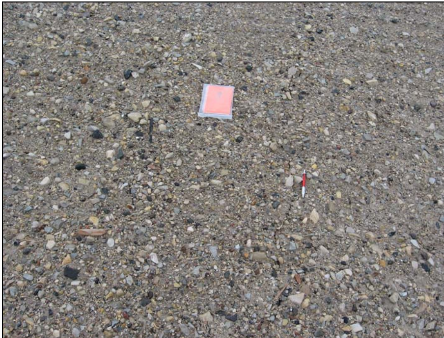
Photograph 8. Close-up photo. Continuing to tracking the tension crack westward along the toe. The pens bracket two tension cracks. The upper crack ends and lower crack continues with a 0.6m offset. ↑
