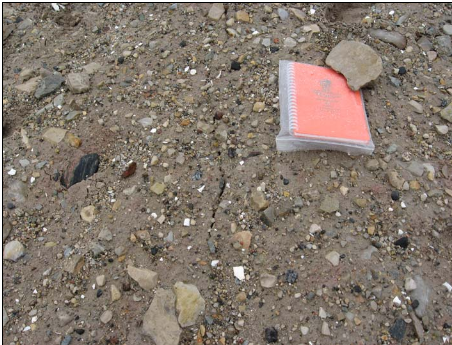
Photograph 16. Close-up of tension crack observed in Photo 15. ↑
