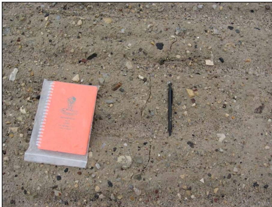
Photograph 14. Fine tension crack about 10 m upslope from the wider crack noted in Photo 13. The crack is parallel to the slope and suggests entire slope may be moving. ↑
