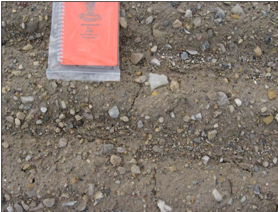
Photograph 10. Tension crack appears to end, possibly infilled with sediments, about 4m up from toe of slope. ↑
