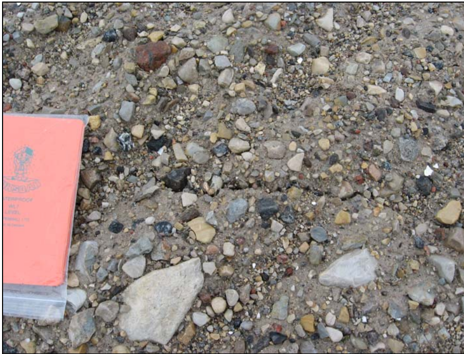
Photograph 6. Close-up of typical crack at NE corner 5m up-slope. Crack fades in and out as some fines have washed in, completely filling some portions of the thin crack. ↑
