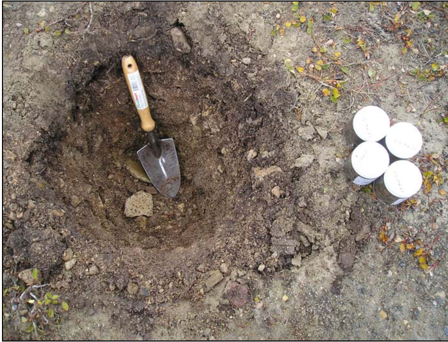
Photograph 3. Test Pit C2-MW-3. Samples C2-MW-3-1 and C2-MW-3-2 collected. ↑
