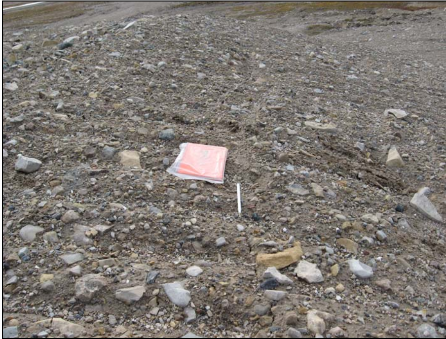
Photograph 7. Tension crack ends about 7m from the NW corner about 1m from top of crest. Field book at end of crack. ↑
