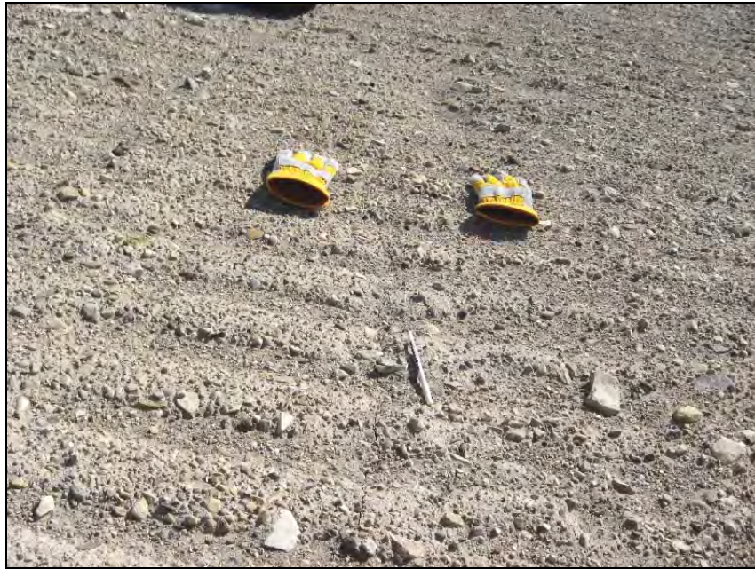
Photograph NH-9. Close-up of crack from last year, partially in-filled with no sign of recent movement (gloves and pen for scale). Splays and offset by up to 1m, always fine. ↑
