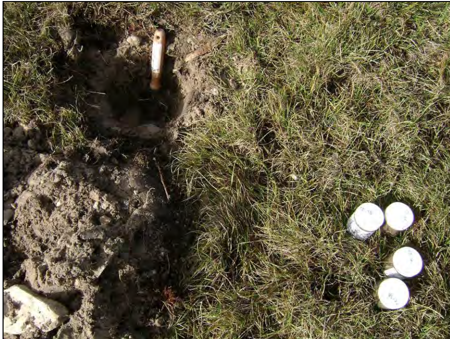
Photograph 3. Test pit at C2-3. Samples C2-3A and C2-3B collected. Water table at 0.40m.↑
