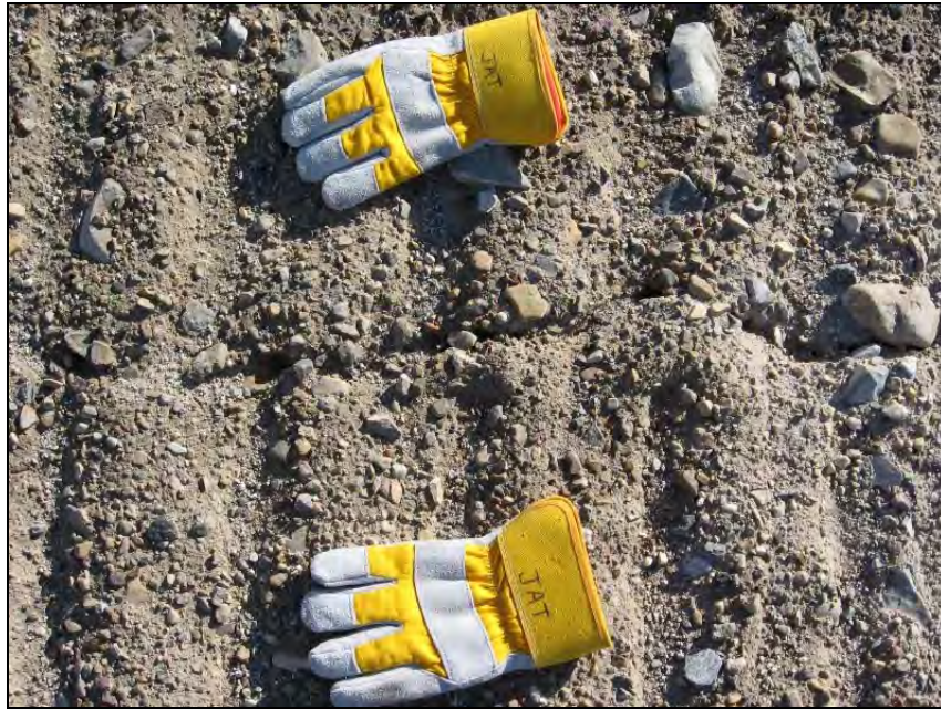
Photograph T2-29. Close-up of crack between gloves. Partially infilled, no sign of recent movement. ↑
