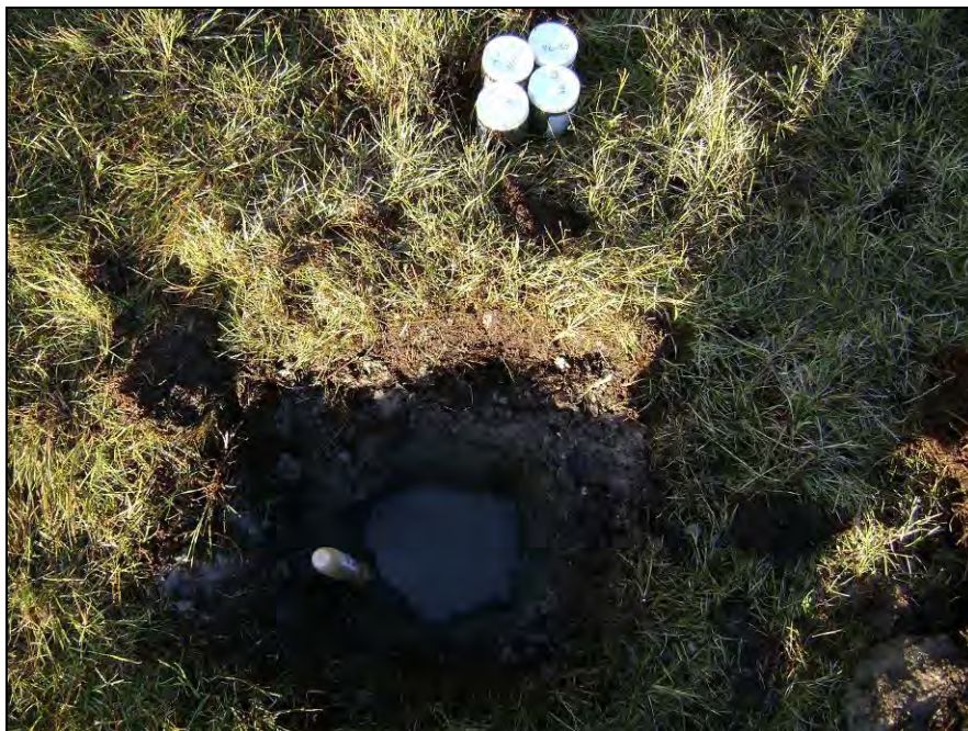
Photograph 2. Test pit at C2-7. Samples C2-7A and C2-7B collected. Water table at 0.30m. ↑
