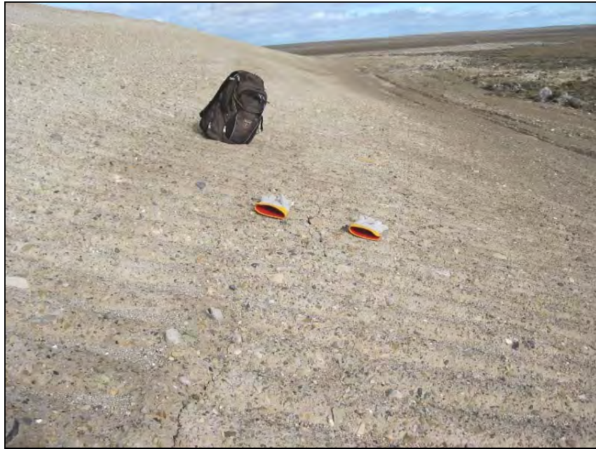
Photograph NH-11. Looking ENE along slope along old, partially in-filled crack (between gloves). ↑
