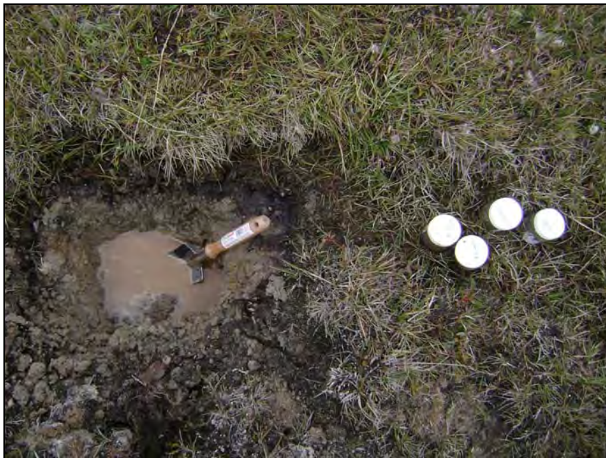
Photograph 8. Test pit at MW-8. Samples C2-MW-8A and C2-MW-8B collected. Water table at 0.20m. ↑
