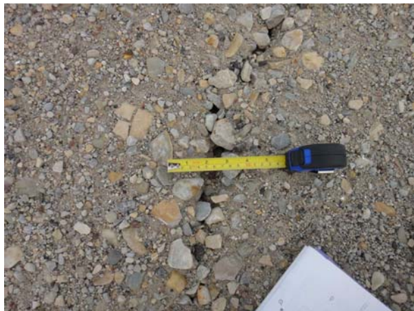
ELLF-17: (left) View looking east-southeast at partially infilled tension crack on southeast cover (Feature B)
