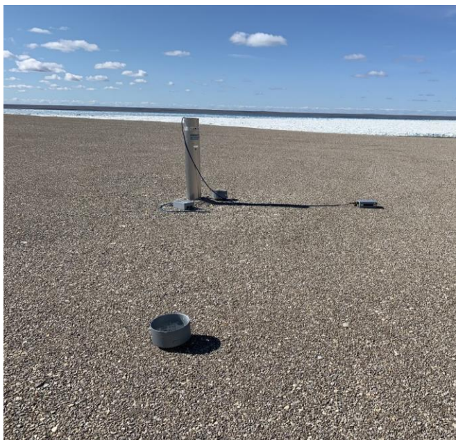
Photograph 2: VT-B-1 Pulled from Casing with VT-B-2 Severed Nearby
