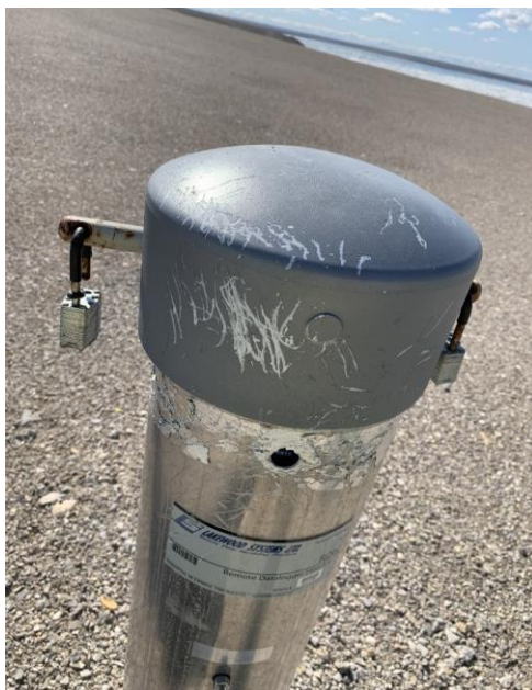
Photograph 1: Evidence of Polar Bear Claw Marks on Thermistor Casings
