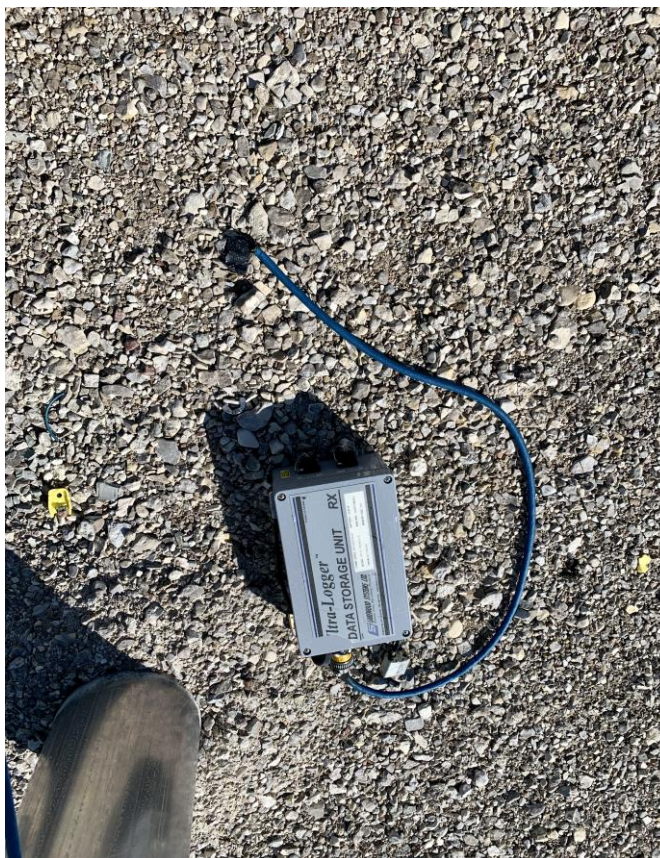
Photograph 3: Severed Data Logger (VT-B-2)
