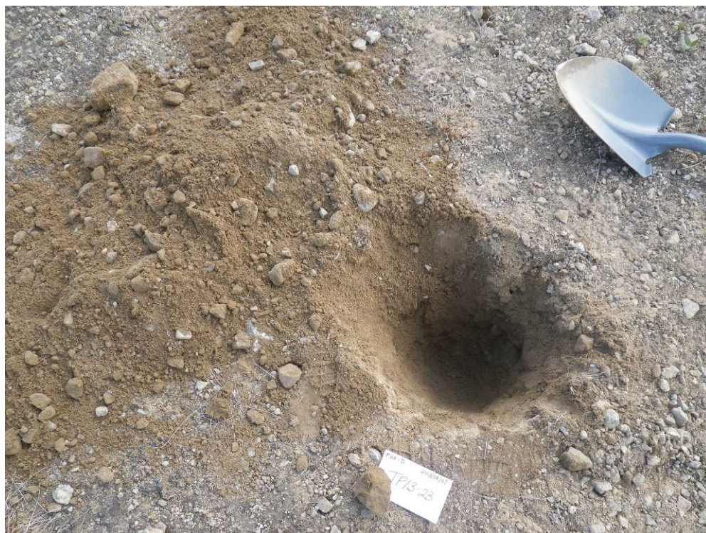
Photo 3 - Typical material used to construct road. TP23 (Station 5+800).
