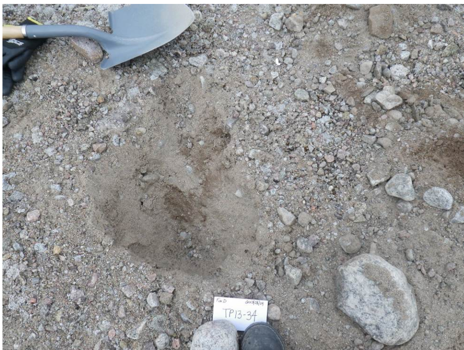
Photo 13 - Typical material used to construct airstrip (TP34).
