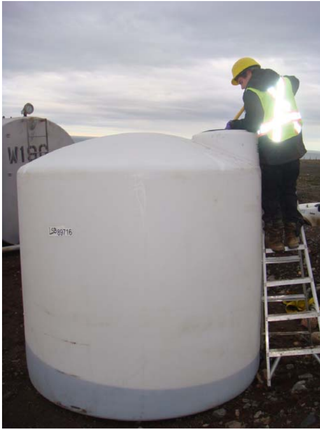
Photo 4 (IMG 2447) Sample 10-16126/16224 Fox-2 Sampling consolidated and treated chlorinated wastewater from fuel tanks in the Beach Refuel Area
