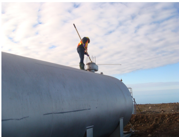
Photo 6 (IMG 2489) Sample 10-16557 Fox -2 Sampling consolidated and treated wastewater from fuel tank W19F in the Beach Refuel Area
