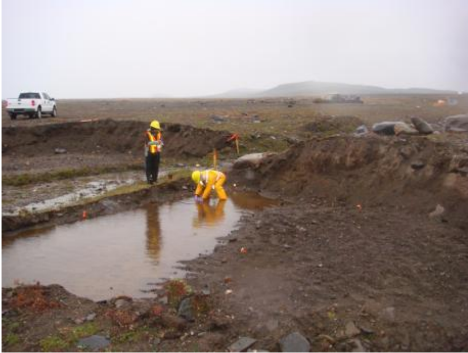
Photo 1 (IMG 2225) Sample 10-15340/41 Fox- 2 Sampling Airstrip South Debris Area Lobe A2 water which had accumulated within the excavation
