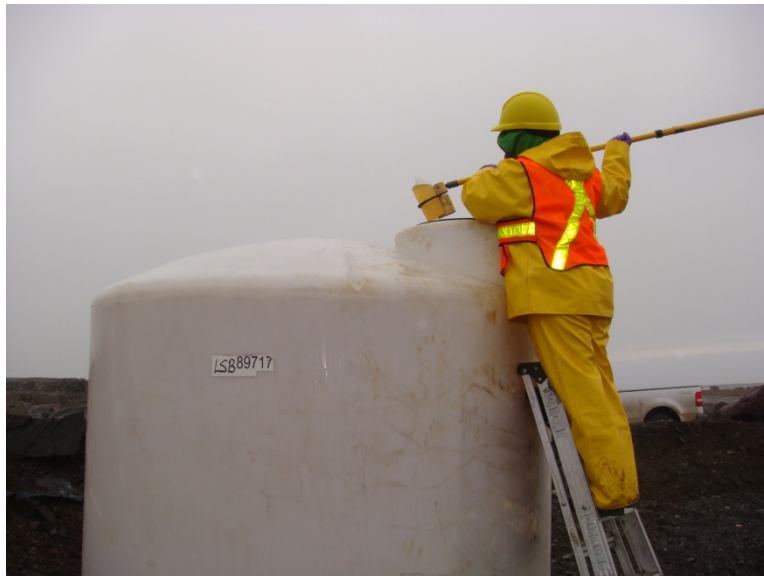
Photo 3 (IMG 2445) Sample 10-16127 Fox-2 Sampling wastewater used to steam clean barrels in the Barrel Processing Area
