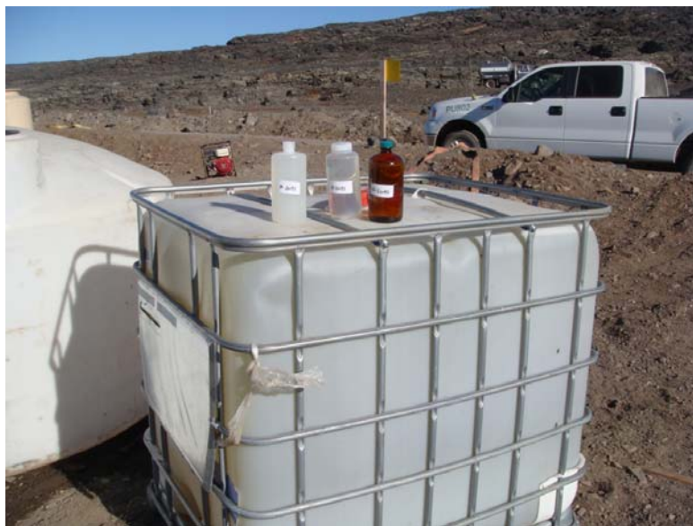
Photo 1 (IMG 2609) Sample 10-20197 Fox-2: Sampling treated water in the cube storage tank within the Temporary Tank Storage Area.
