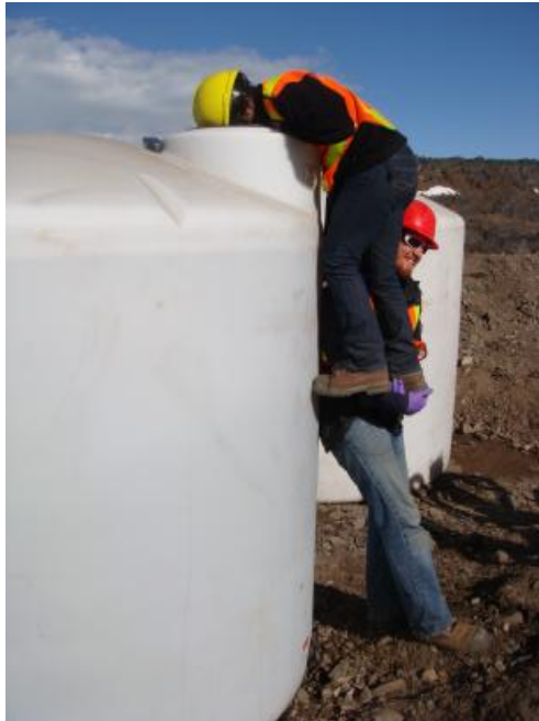
Photo 4 (IMG 2115) Sample 10-14588 Fox-2 Sampling the tank of containerized contact water from ASL Lobe A.
