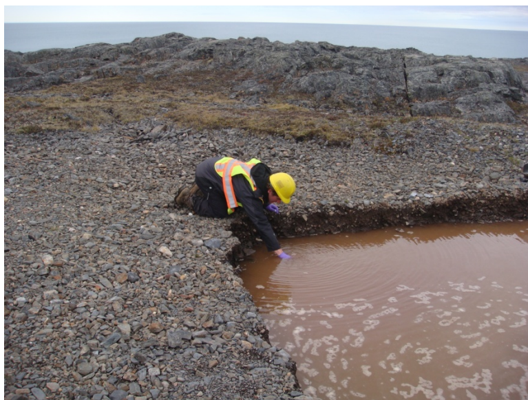
Photo 5 (IMG 2450) Sample 10-16129 Fox-2 Sampling wastewater from WL-18297 which had accumulated after excavation
