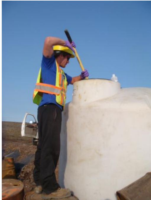
Photo 2 (IMG 2311) Sample10-15400/01 Fox 2- Sampling wastewater from barrels consolidated and treated in Tank III in the Barrel Processing Area
