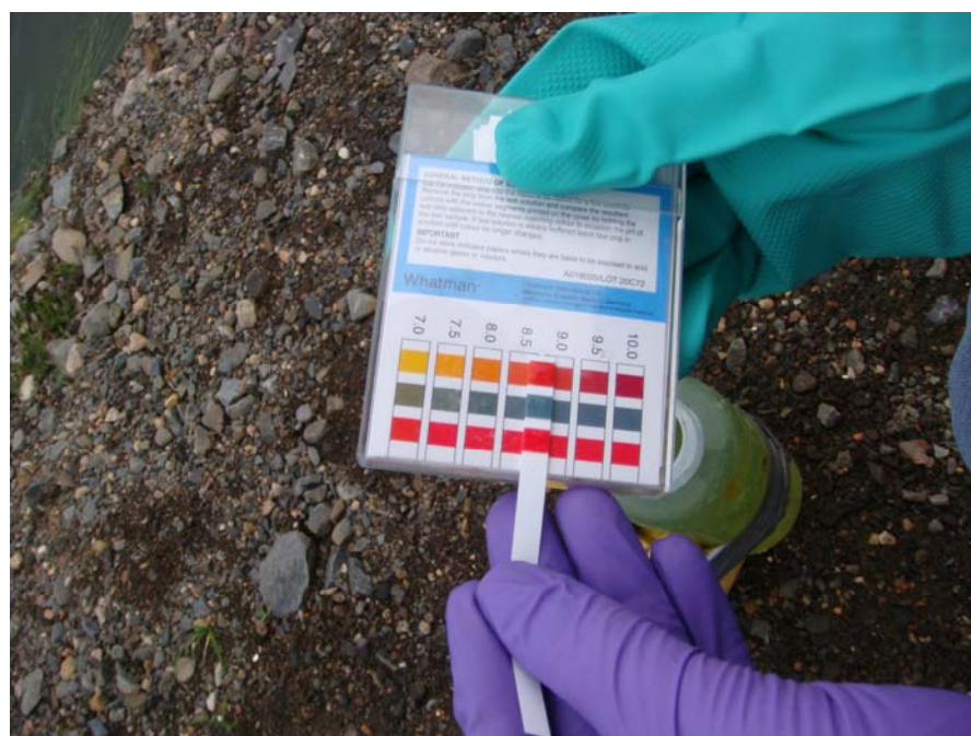
Photo 3: Close up of indicator paper used to test the pH of sewage lagoon cell 3. The indicator paper specifies a pH of 8.0 to 8.5. The photo was taken at the time of testing on July 21 st .
