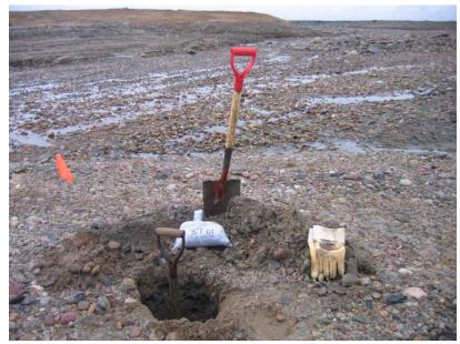
Photo 16: Test Pit at Borrow Source #7
