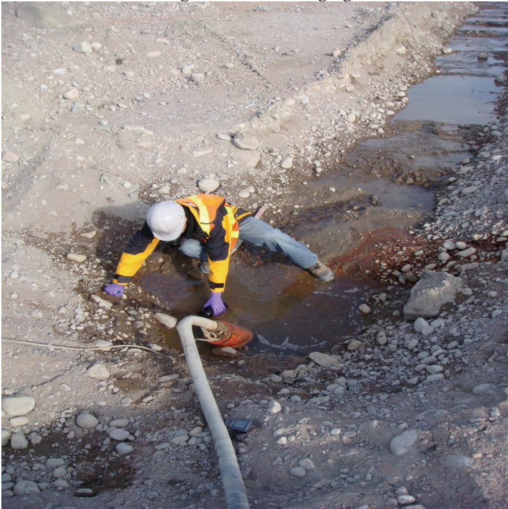
Photo 5 (DSC00746): Sample 09-17599 east along the trench dug for removing upwelling groundwater in the landfarm. The area is also bermed off to prevent any surface water from the landfarm from entering into the discharging water.
