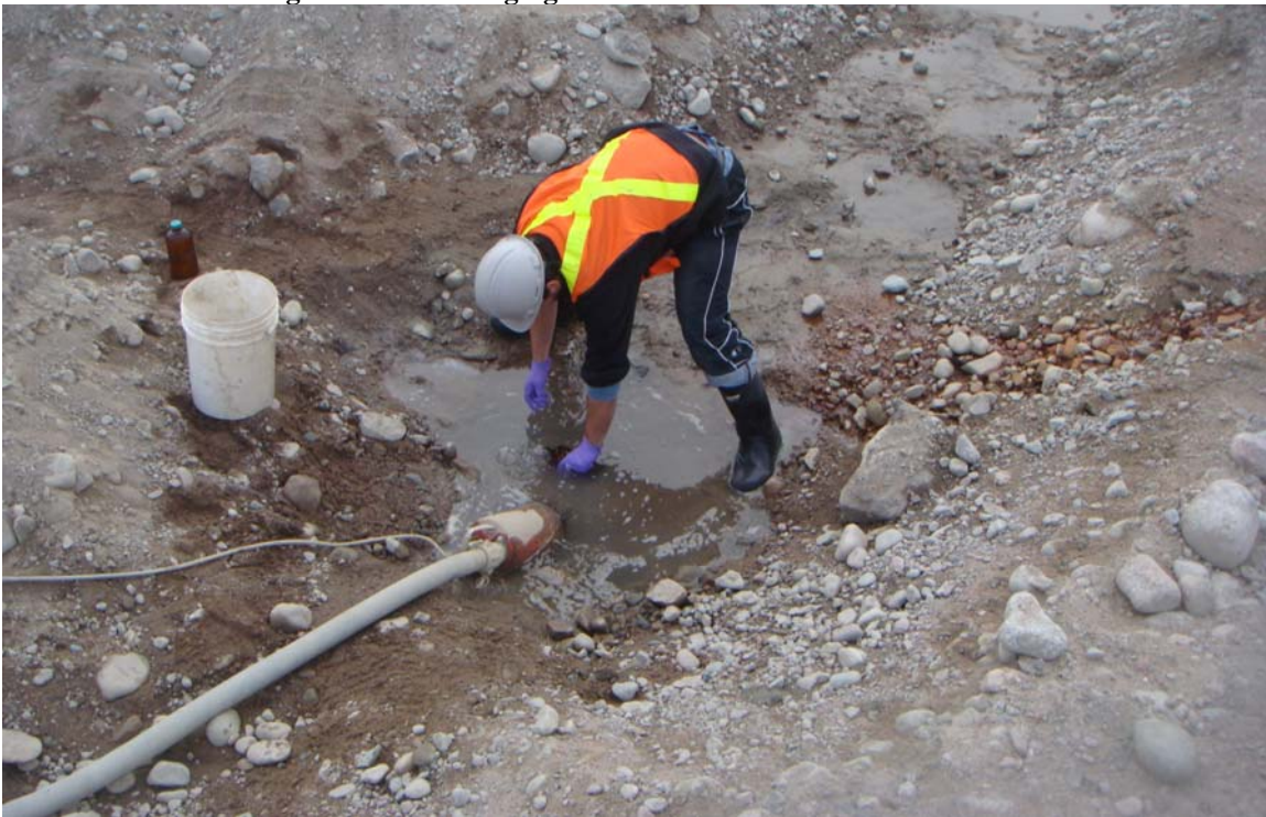
Photo 6 (DSC01620): Sample 09-22271 and 09-23816 photo is taken from the top of the western berm of the land farm looking east along the trench dug for removing upwelling groundwater in the landfarm from entering into the discharging water.
