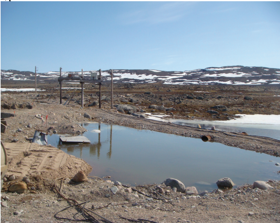
Photo 2 (DSC01397): Sample 09-16390 and 09-16391 water pooling over contaminated soil area AA-1, photo faces south west.
