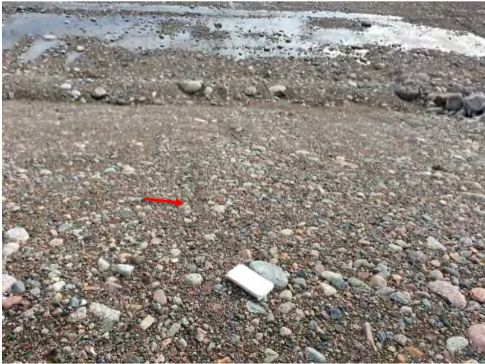
Photo 99: Non-Hazardous Waste Landfill- South slope, Feature I-Self-armouring erosion, facing southeast (Acceptable) (CAM5_Photo34.jpg)
