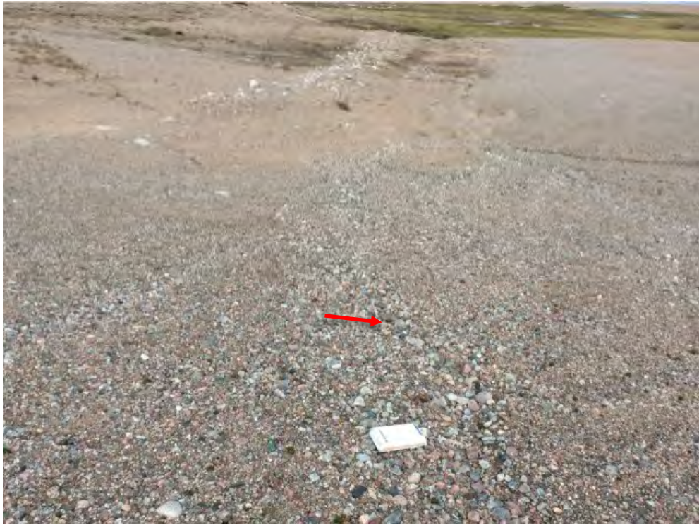
Photo 63: Lower Site Landfill South- Northwest slope, Feature AB—Minor self-armouring erosion, facing north (Acceptable) (CAM5_Photo92.jpg)
