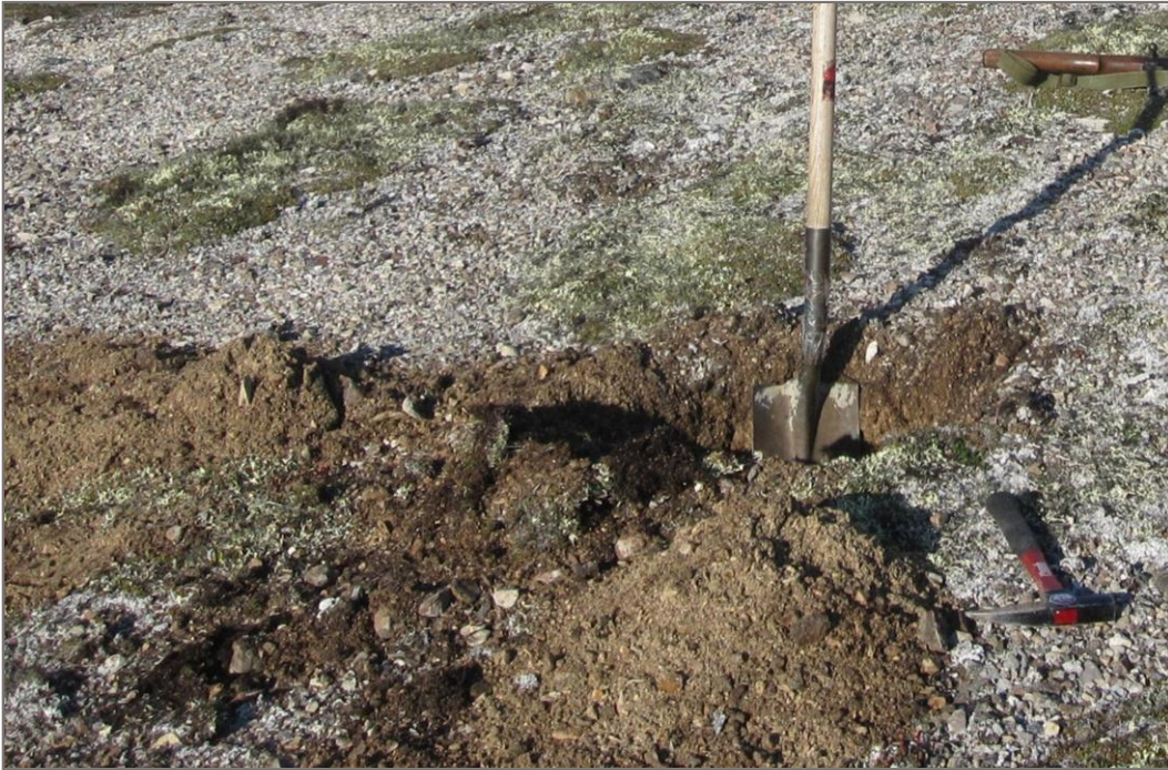
Photo G5: Gravelly sand with a trace of fines and 30-40% calcareous material at Borrow B
