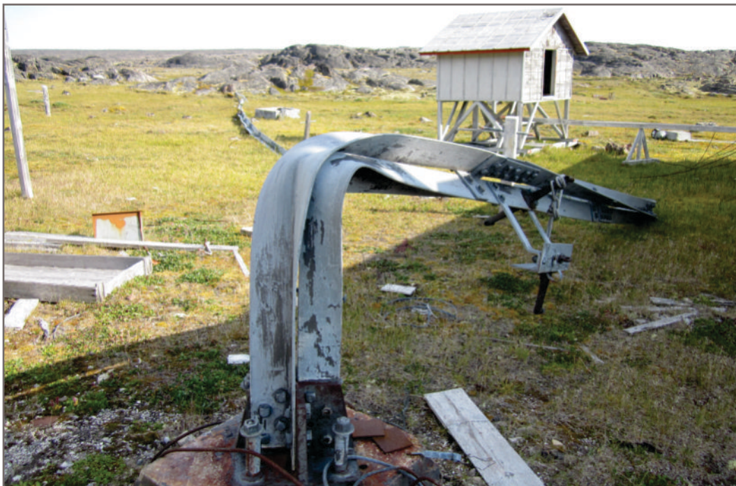
Photo H-6: Total and leachable lead paint on fallen metal pole adjacent to the New Radio Building, various poles were found on-site
