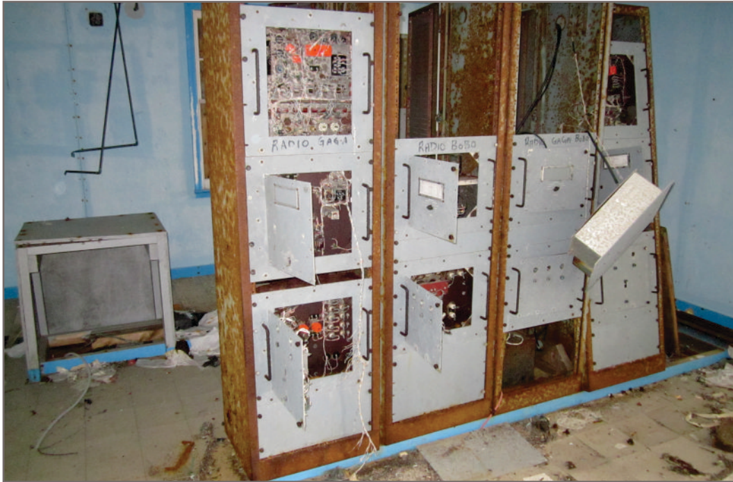
Photo H-5: Example of mercury, PCBs and lead solder in electrical components, and total and leachable lead paint on metal (APEC 3 - New Radio Building shown)
